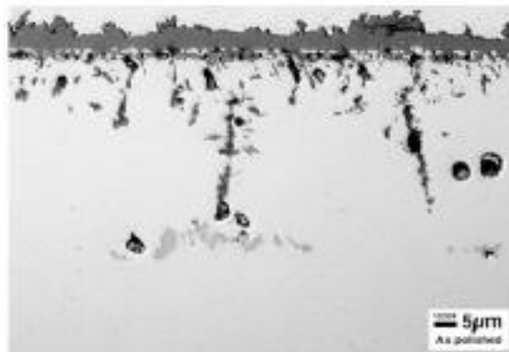
Figure 2-37 Scaled developed on Inconel 617 after 4000 hour exposure at 800°C in 17 bar steam [23]
