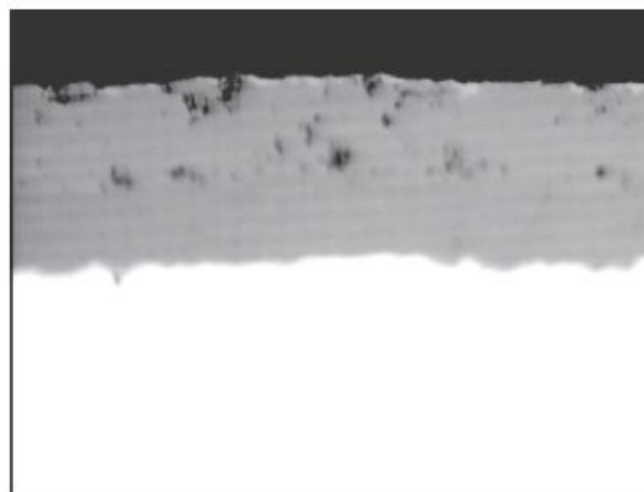
Figure 2-26 The scale formed on the T22 ferritic steel at 550°C [72]
