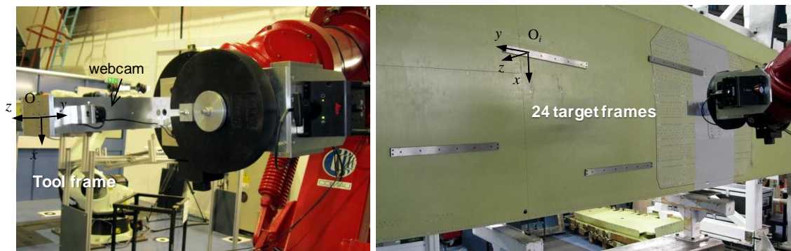
Figure 8-18 In the demonstration, the robot must align the tool frame with 24 target frames located on a stabilizer structure
