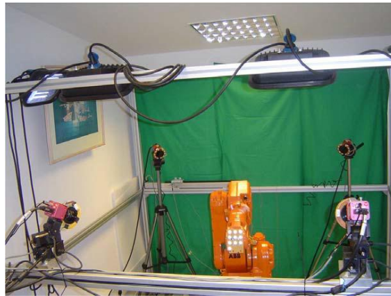
Figure 3-8 The visual-servoing demonstrator of the ARFLEX project (ARFLEX, 2011)
