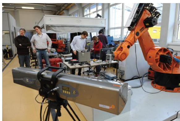
Figure 2-17 The K-series Optical CMM (photogrammetric system) is used for tracking the position of a KUKA robot (Nikon Metrology)
