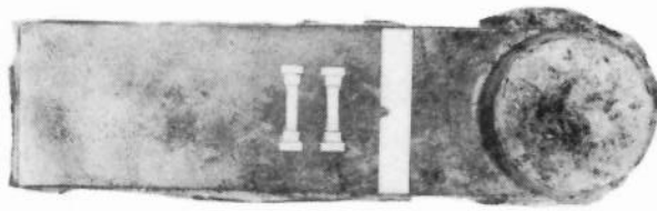
FIGURE 8. PHOTOGRAPH OF DUMMY TEST CASTING SHOWING POSITION OF TEST PIECES.
