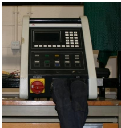
Figure 5.9 EDF Minac Twin 20/40 induction heaters used in TTH induction heating experiments
