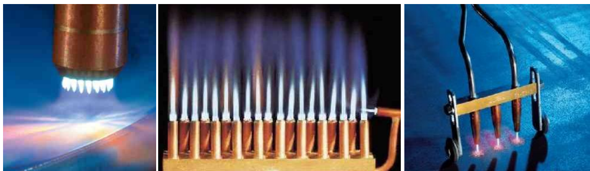
Figure 2.11 Different oxy-acetylene heating and air-acetylene torches [27, 28]
