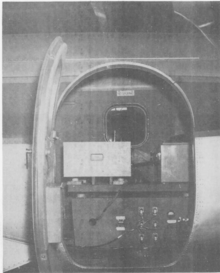
ELLIOT 10-CHANNEL STRAIN GAUGE RECORDER FOR NOSE \frac{U}{C} LOAD MEASUREMENT
