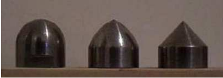
Figure 2-6 Hemispherical, ogival and conical Impact Tups [43]
