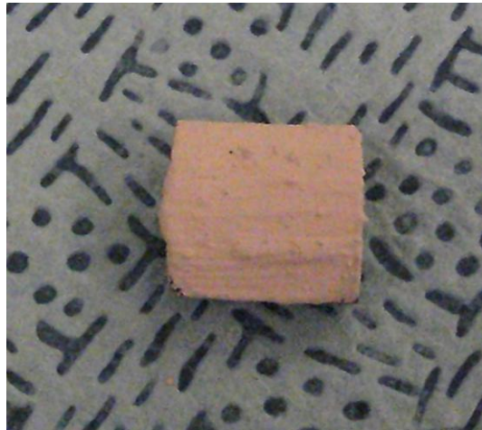
Figure 3-3: Sample covered with deposit prior to heat exposure.
