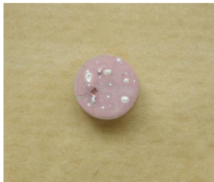
Figure 3-18: Disc with deposit D4 after 200 hours exposure in simulated oxy-fired combustion gas at 650°C
