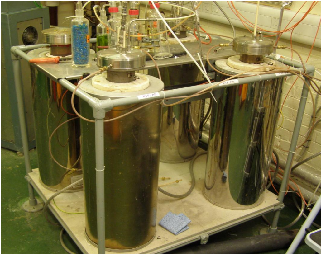
Figure 3-6: A bank of four fireside corrosion vertical furnaces facility at Cranfield University.
