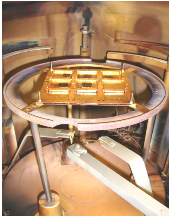
Figure 4.3 View inside the vacuum chamber of the Edwards E480 thermal evaporator showing the position of the metal mask plate relative to the tungsten spiral filament and molybdenum boat.
