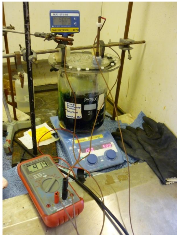
Figure 4.9 Nickel electroplating facility (plating bath, heater/stirrer unit, and multimeter). The DC current supply unit is not shown.
