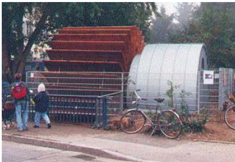
Figure 28 Modern waterwheel installation in Germany (Davison and Bacon, 2004)
