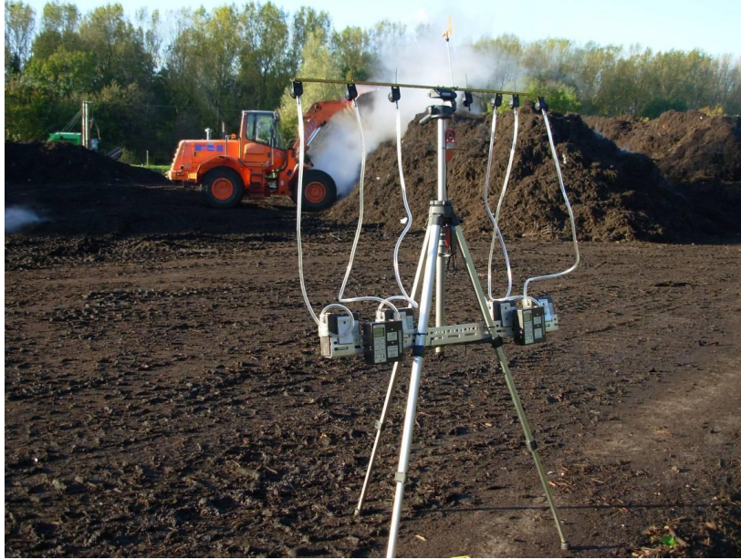
Figure 3.3: Photograph of sampling set-up detailed in Figure 3.1; compost turning visible in background. Taken on the 17 th October 2007 at Lount OWC.
