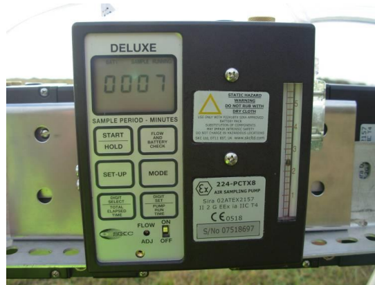
Figure 3.4: SKC PCXR8 personal sample pump
