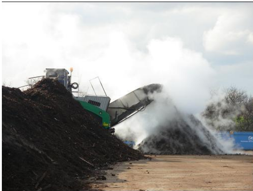
Figure 2.10: Turning using a dedicated windrow turning machine at Flixborough
