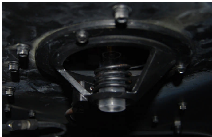
i) RF copper coil, following the machining of a window in the housing.
