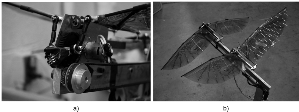
Figure 2.35: Mechanical flapper of Warkentin & DeLaurier (2007); a) details of flapping mechanism; b) assembled flapper
