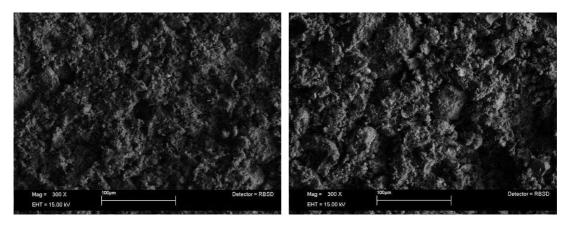
**Figure 5-49a, b.** SEM backscattered electron (BSE) images of examples of red ochres BLN 007 and AMN 005
