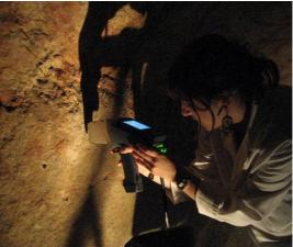
**Figures 4-34a, b.** Collecting XRF data from the ochre wall paintings in the Hal-Saflieni Hypogeum
