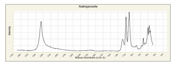
**Figure 4-18.** % Absorbance reference chart of natrojarosite (Downs, 2006)
