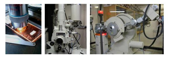
**Figures 4-2a-c.** (a) Observing a dispersed sample (b) The SEM-EDS and (c) an XRD (Photos: author)
