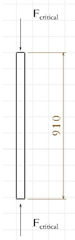
Floor vertical struts
