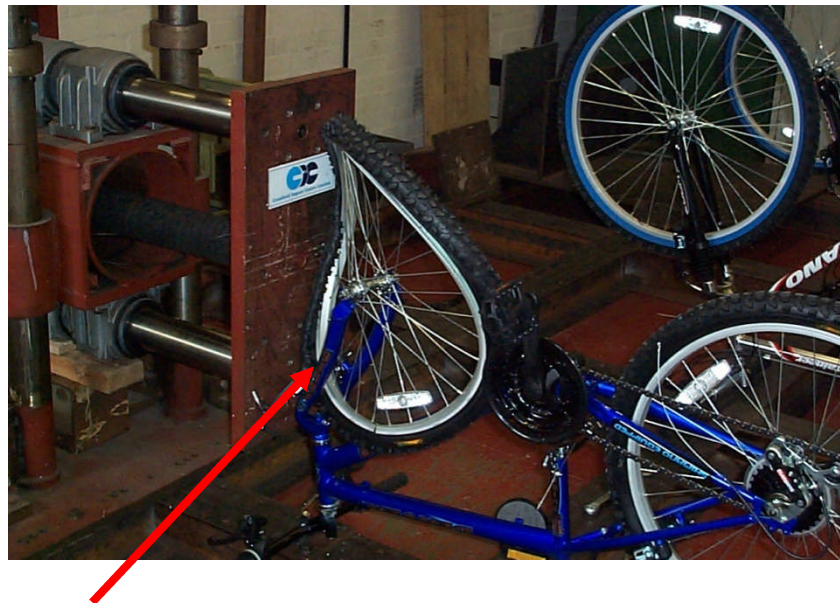
Figure 4-35: Test #3 Showing Deformations of Forks and Wheel Collapse.
