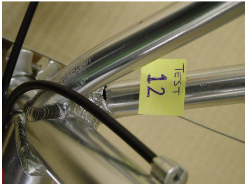
Figure 4-46: Post Test Photograph Showing Split in Aluminium Frame Near Seat Post.
