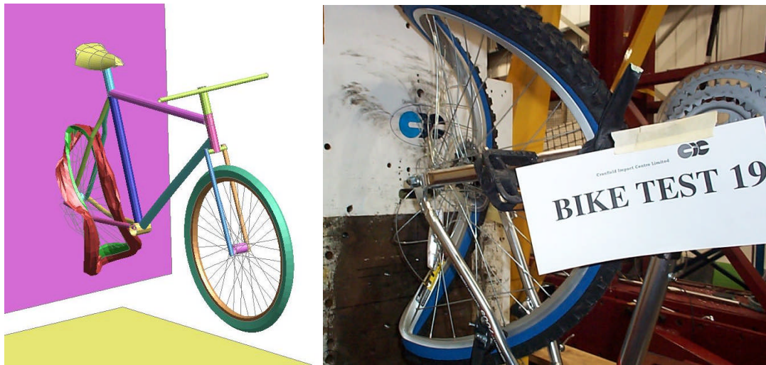
Figure 4-3: Deformed Bicycle from Flat Wall Rear Impact Scenario – Model and Test
