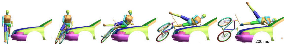
Figure 4-9: Cyclist Struck Leg-Up Kinematics from Impact by the Large Family Car Model
