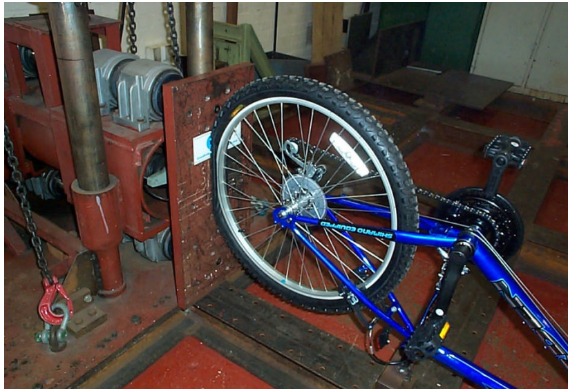
Figure 4-33: Actuator and Platform used for Static Tests.
