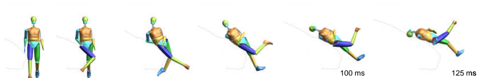
Figure G-15: Pedestrian Struck Leg-forward Kinematics from Impact by the MPV Model
