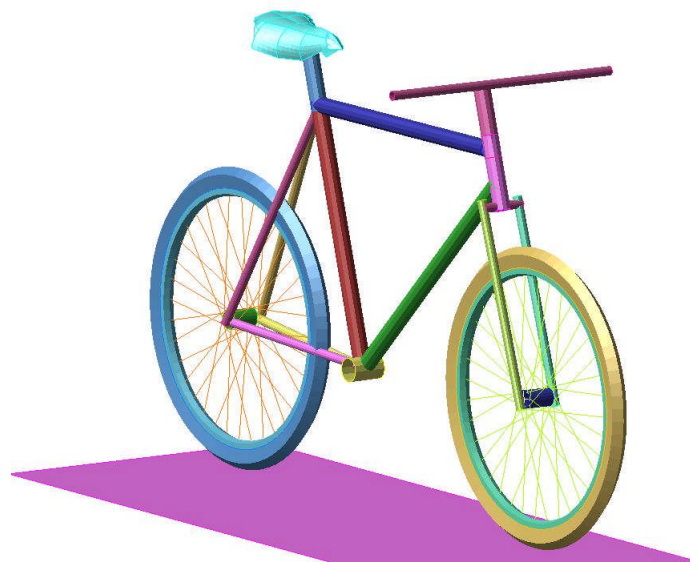
Figure 3-6: Finite Element Model of Adult Bicycle
