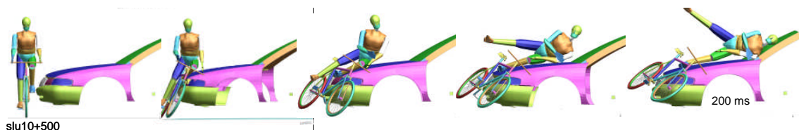
Figure 4-16: Cyclist Struck Leg-Up Kinematics from Impact by the Large Family Car Model with Cyclist Offset +500 mm
