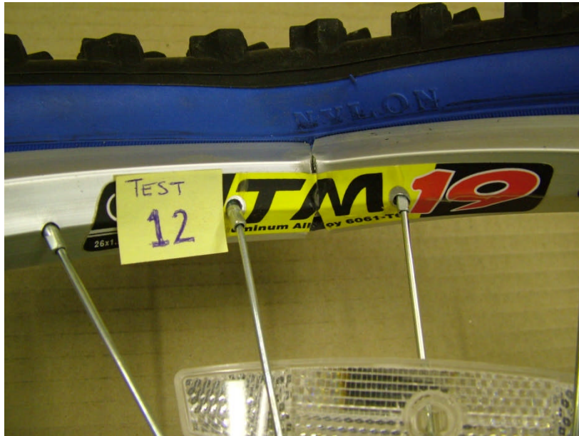
Figure 4-36: Wheel Failure in Adult Bike at Rim Connection Location, Test #12
