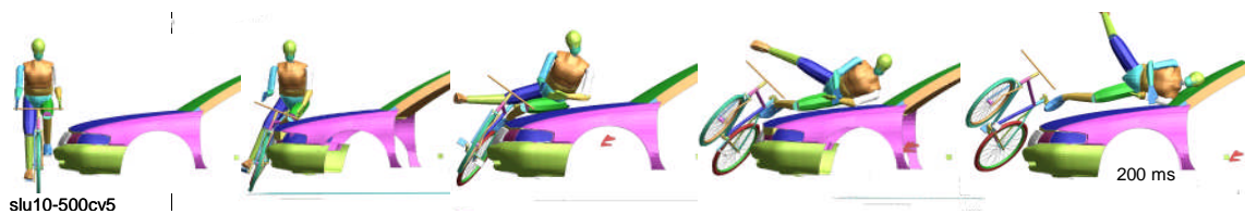
Figure 4-17: Cyclist Struck Leg-Up Kinematics from Impact by the Large Family Car Model with Cyclist Speed of 5 m/s and Offset -500 mm
