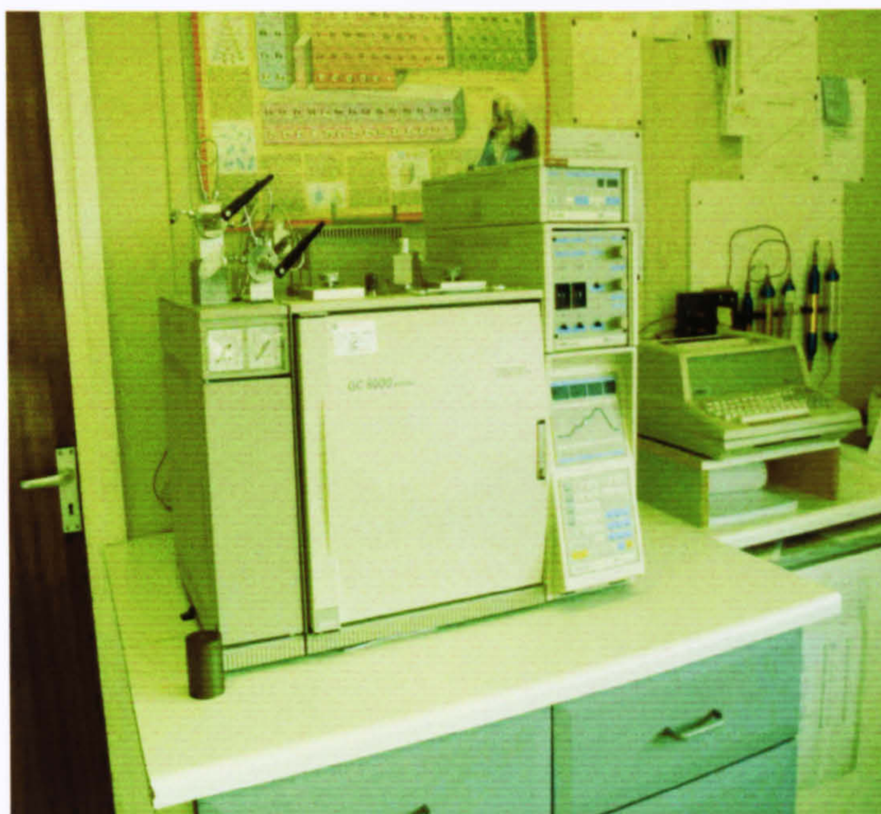
Figure 2.4 Gas chromatograph used for analysing the carbon dioxide and oxygen levels from the outlet tube of each of the nine treatment containers.
