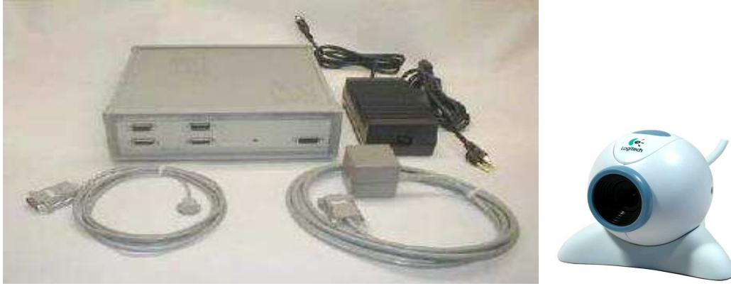
Figure 4.2: Input Devices for FDO gestures. Tracker-based Polhemus FasTrack (left) is used for acquiring for FDO_PT dataset. Whereas for computer vision-based data polling, an average desktop webcam (right) is used. Even though, Polhemus FasTrack provides four sensors, only two sensors are used, each of which is used for a hand.
