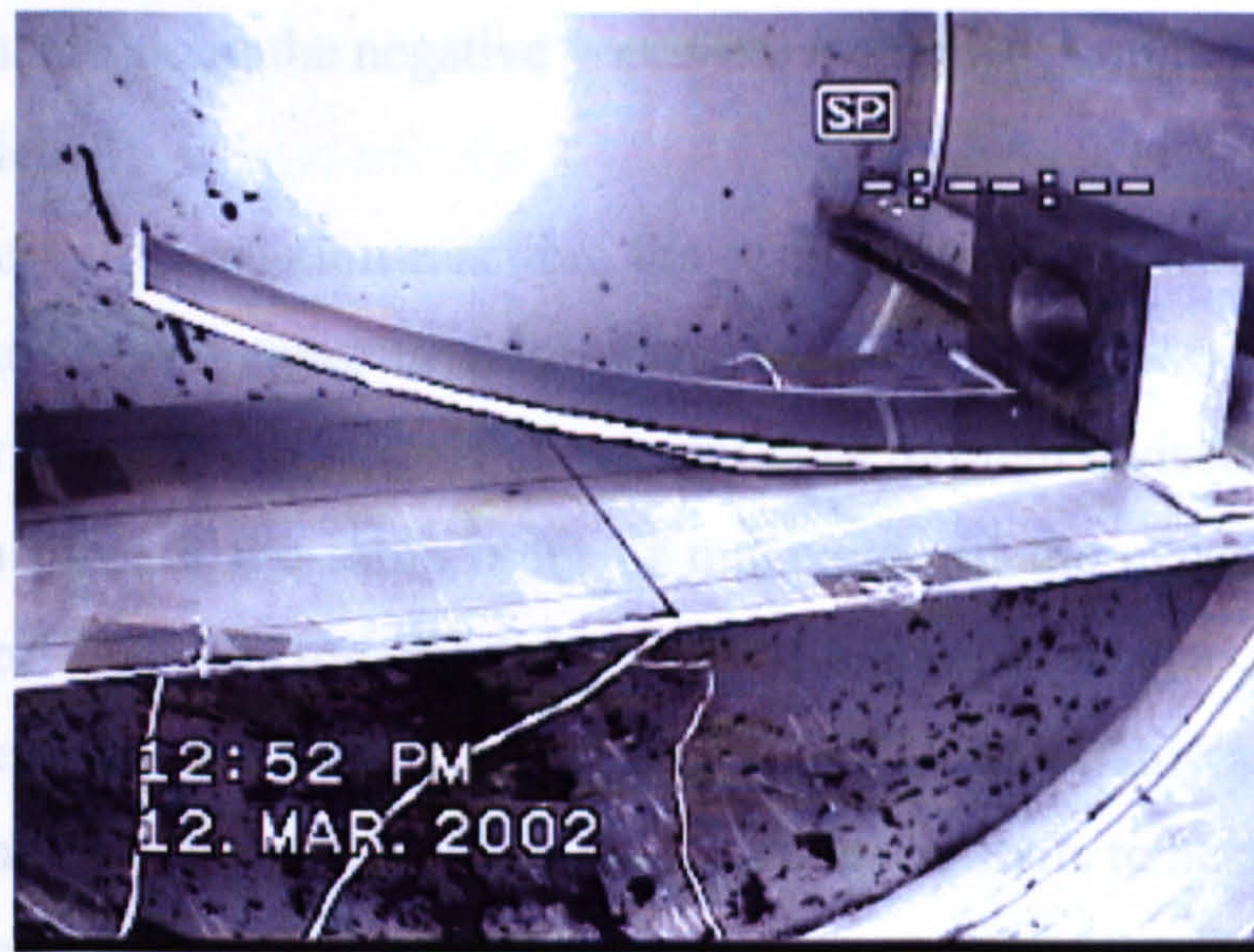
Fig. 9.3 Picture of the bi-material sample on support plate at position 3 (at height h_3 ) in the oven after testing.
