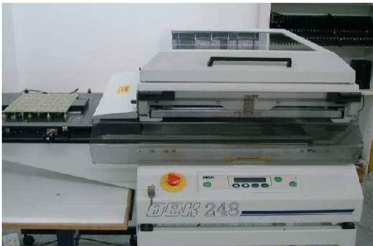
Figure 2.2: The DEK 248 Automated screen-printing machine used for manufacturing the SPEs.
