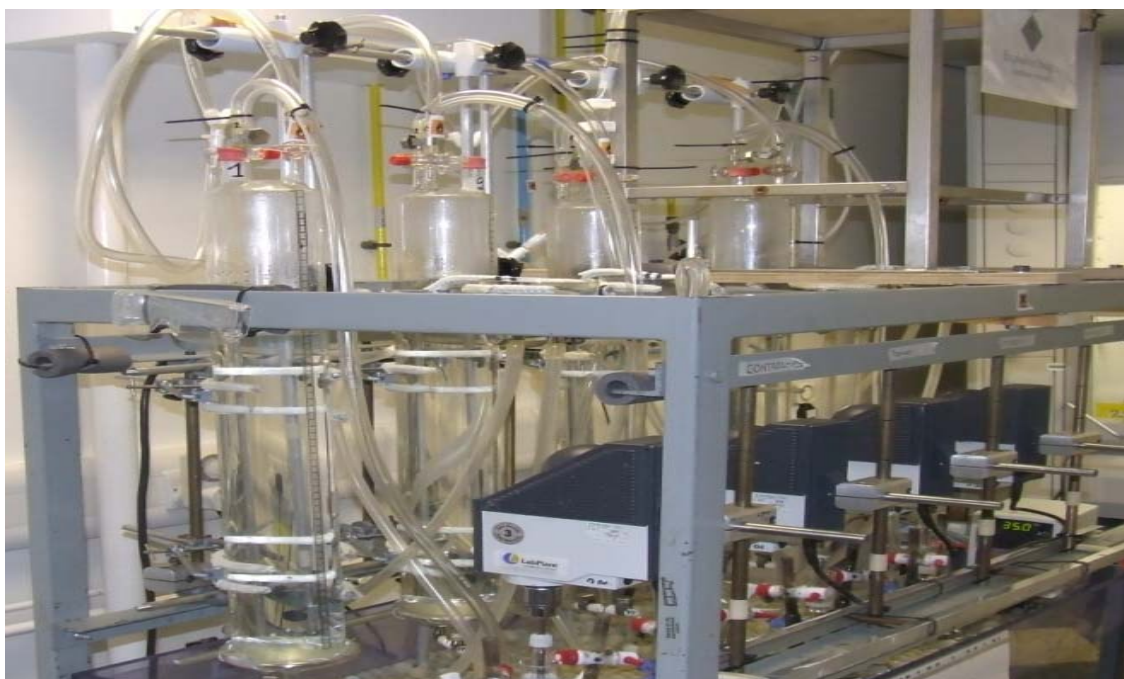
Figure 3-3 Gas measuring apparatus of the lab scale anaerobic digesters.
