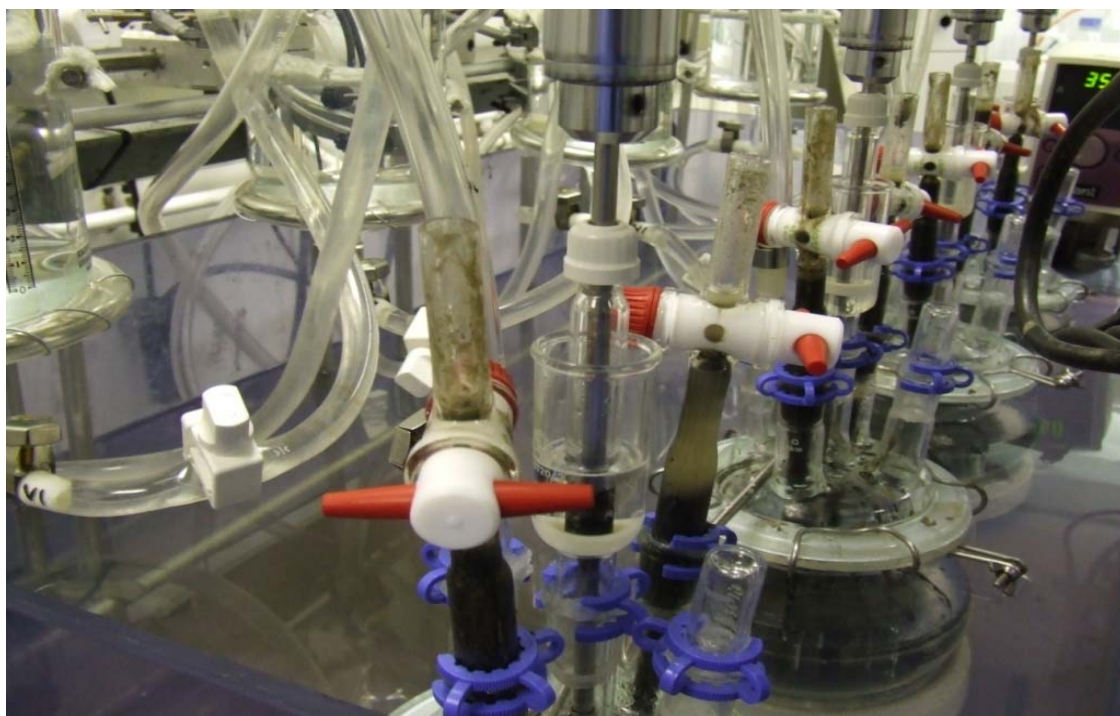
Figure 3-2 Setup of anaerobic digesters/bioreactors.
