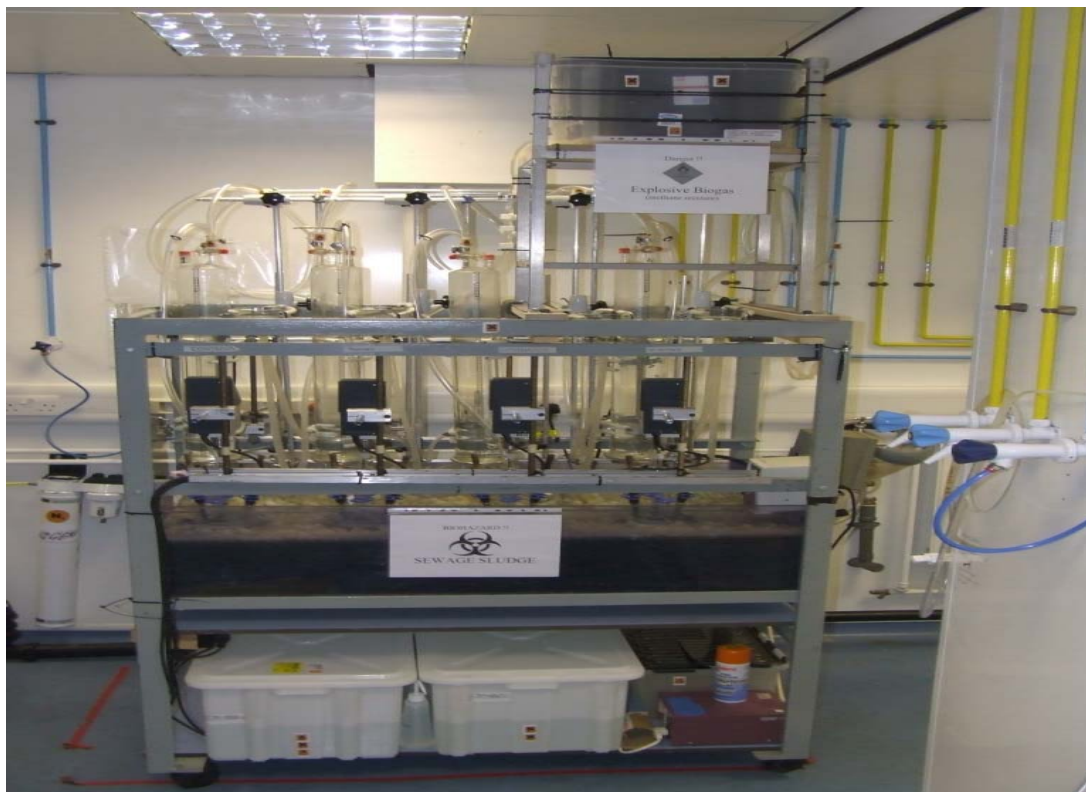
Figure 3-4 Lab scale anaerobic set up used for the evaluation of EDCs.
