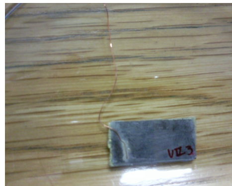
(d) Typical laminate composite sample with an electrical wire attached
