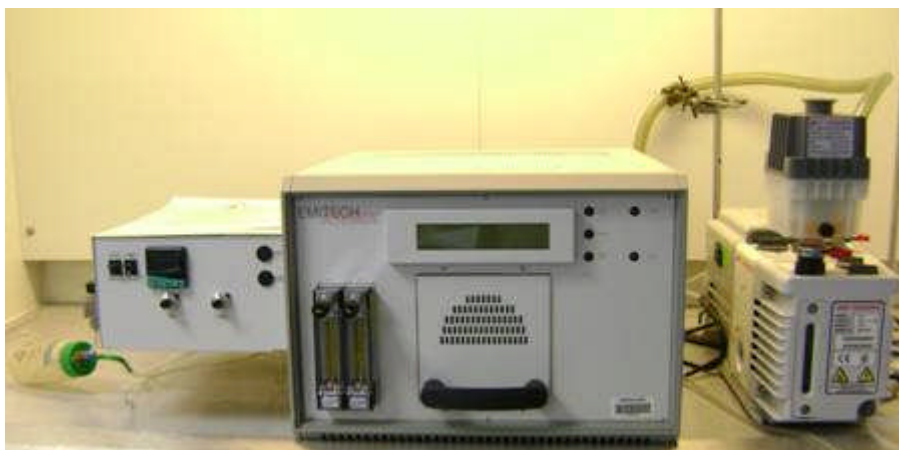
Fig. 3.4. Plasma chamber (Emitech) with integrated Liquid and Gas Controllers (Horiba).
