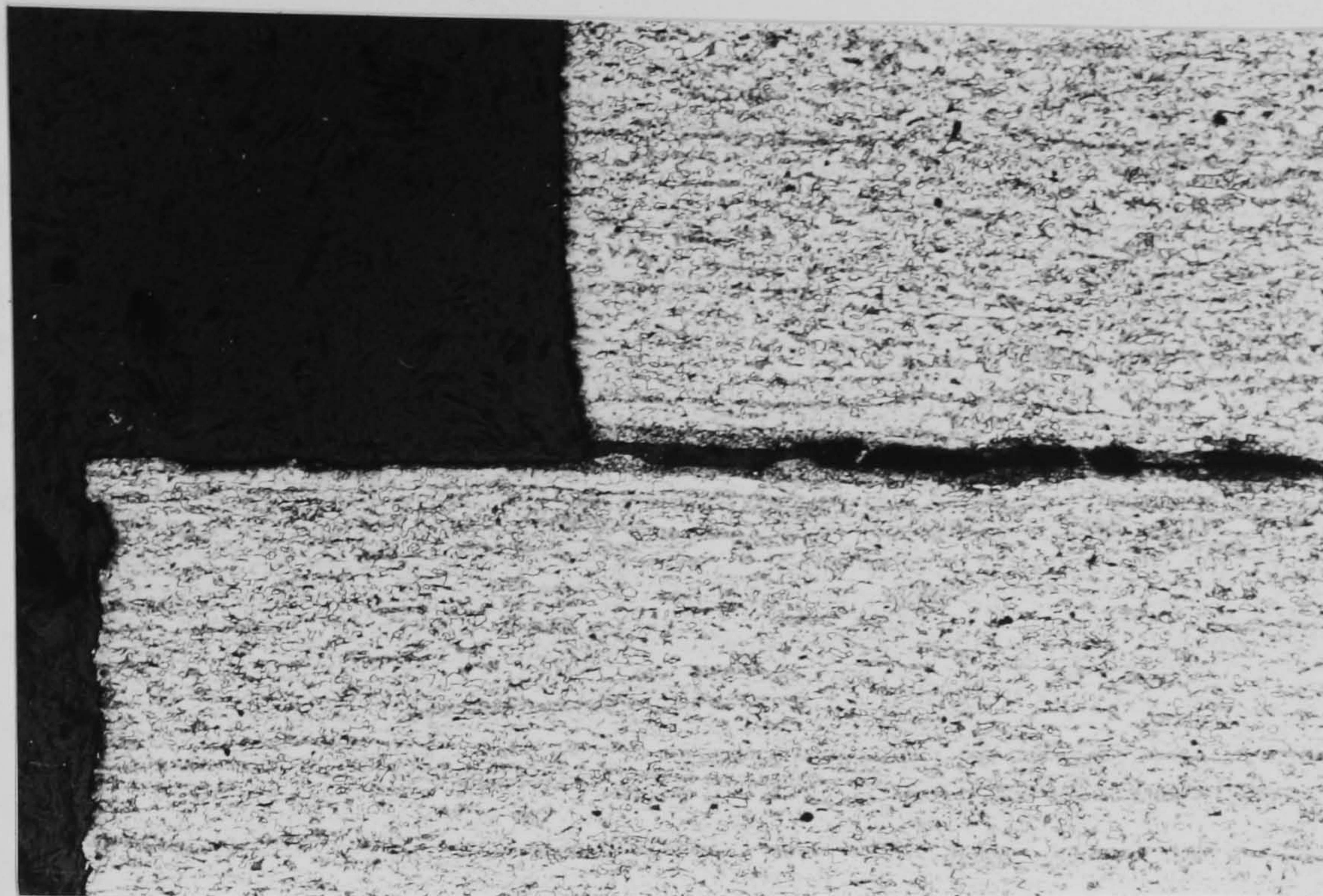
Figure 86 Local microstructure associated with delamination in profile (x200).
