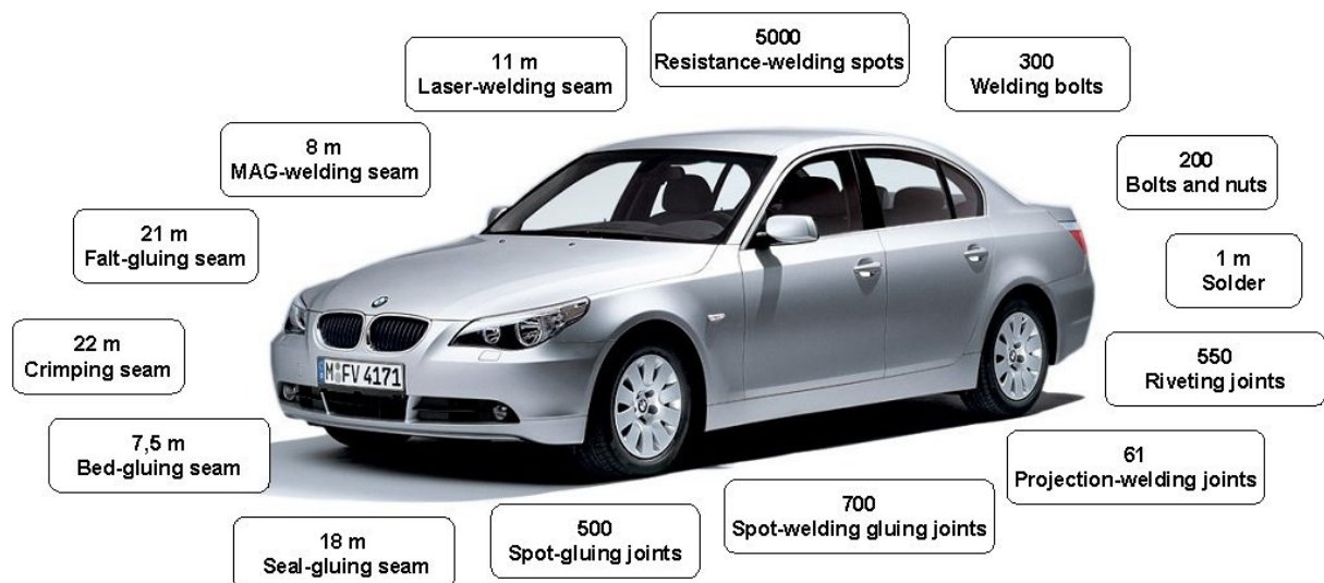
Figure 2.4: An example of the number of JT's for the BMW 5-series [Witte, 2000].
