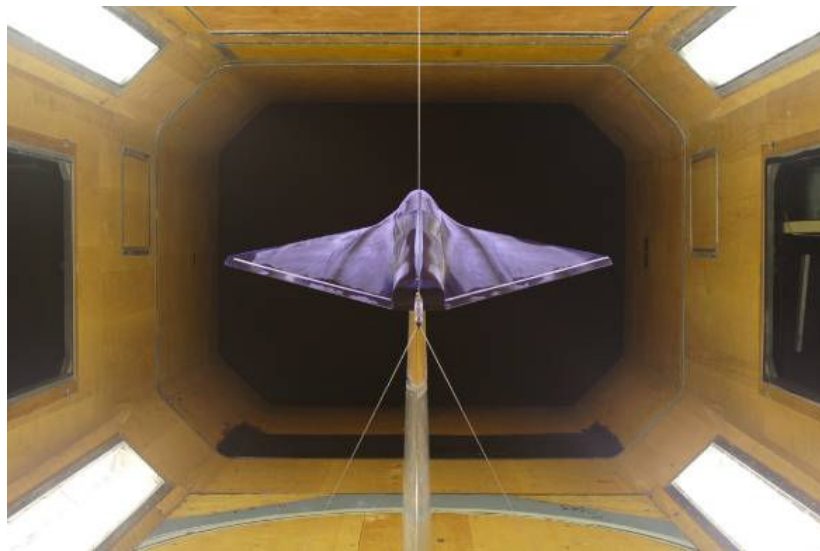
Fig. 3-3. 50% scale full-span DEMON model mounted in the 8x6 foot wind tunnel at Cranfield University. (Downstream/back view, image was rotated through 180°)
