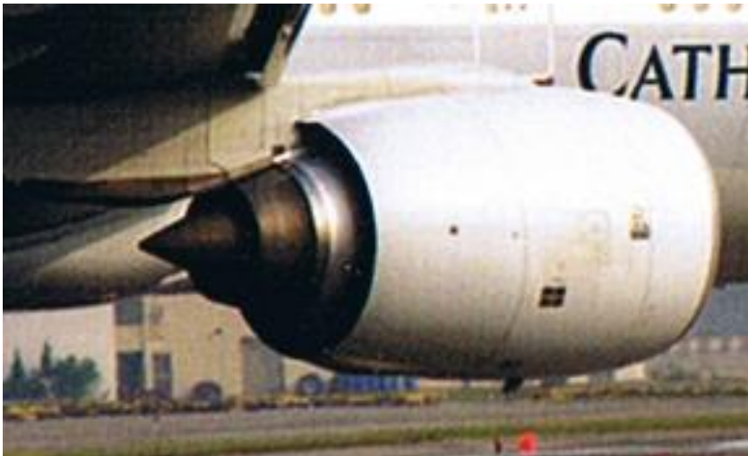
FIG 3.1.16 COWLING OF RR TRENT 892 POWERPLANT SHOWING PROTRUDING TAIL CONE Image Courtesy Rolls- Royce
