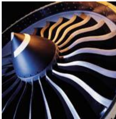
FIGS 3.1.1 TYPICAL MODERN (2008) AERO ENGINE FAN SHAPES (REFS [3.3] AND [3.4] RESPECTIVELY)
