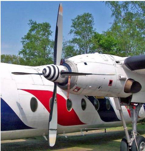
FIG 3.6.1 ROLLS-ROYCE DART ENGINE MOUNTED ON FOKKER F27 [3.68]
