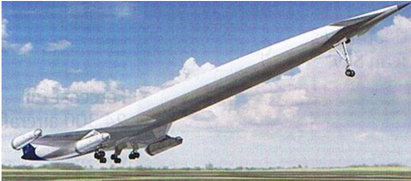
FIG 4.0.3 MACH 5 AIRLINER PROJECT [4.4]
