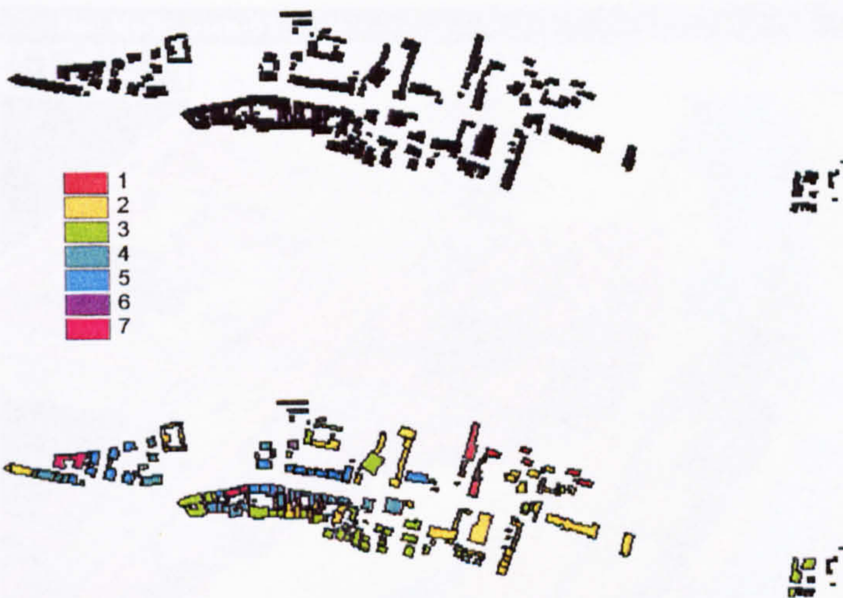
(scaled and geo-referenced aerial image overlaid with the built form as closed polygon data set – shown as figure ground image and as coded polygons based on number of storeys)
