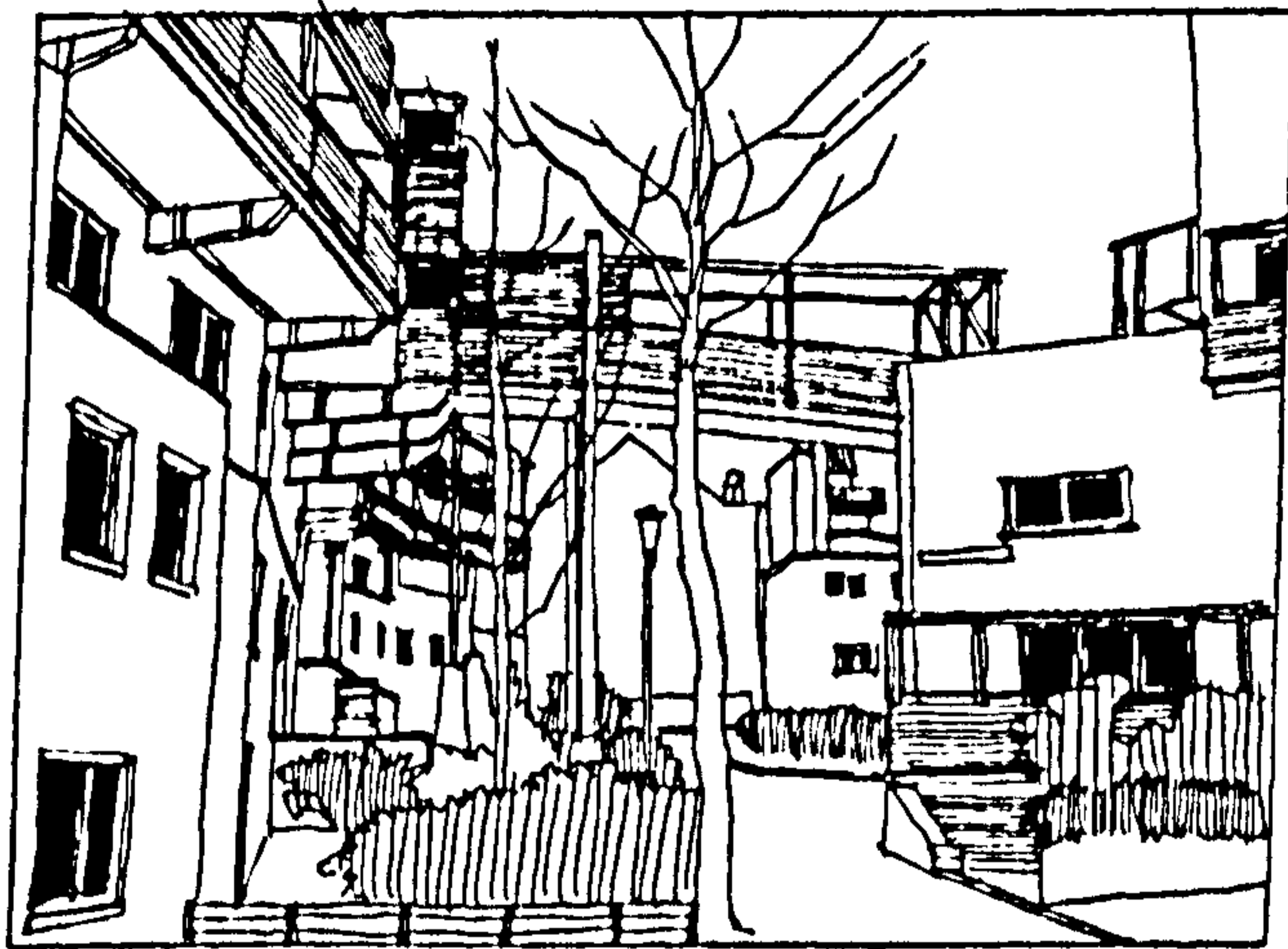
(The unresilient 'Tyneside flats' (left) that remain in Byker. What appears to be terraced houses, is actually ground and first floor flats at a high density – note double the expected number of doors. These were replaced by a flexible block (below) – the Wall – designed to be able to be adapted and sub-divided both horizontally and vertically to provide a range of accommodation, from one bedroom flats to five bedroom family homes.)
