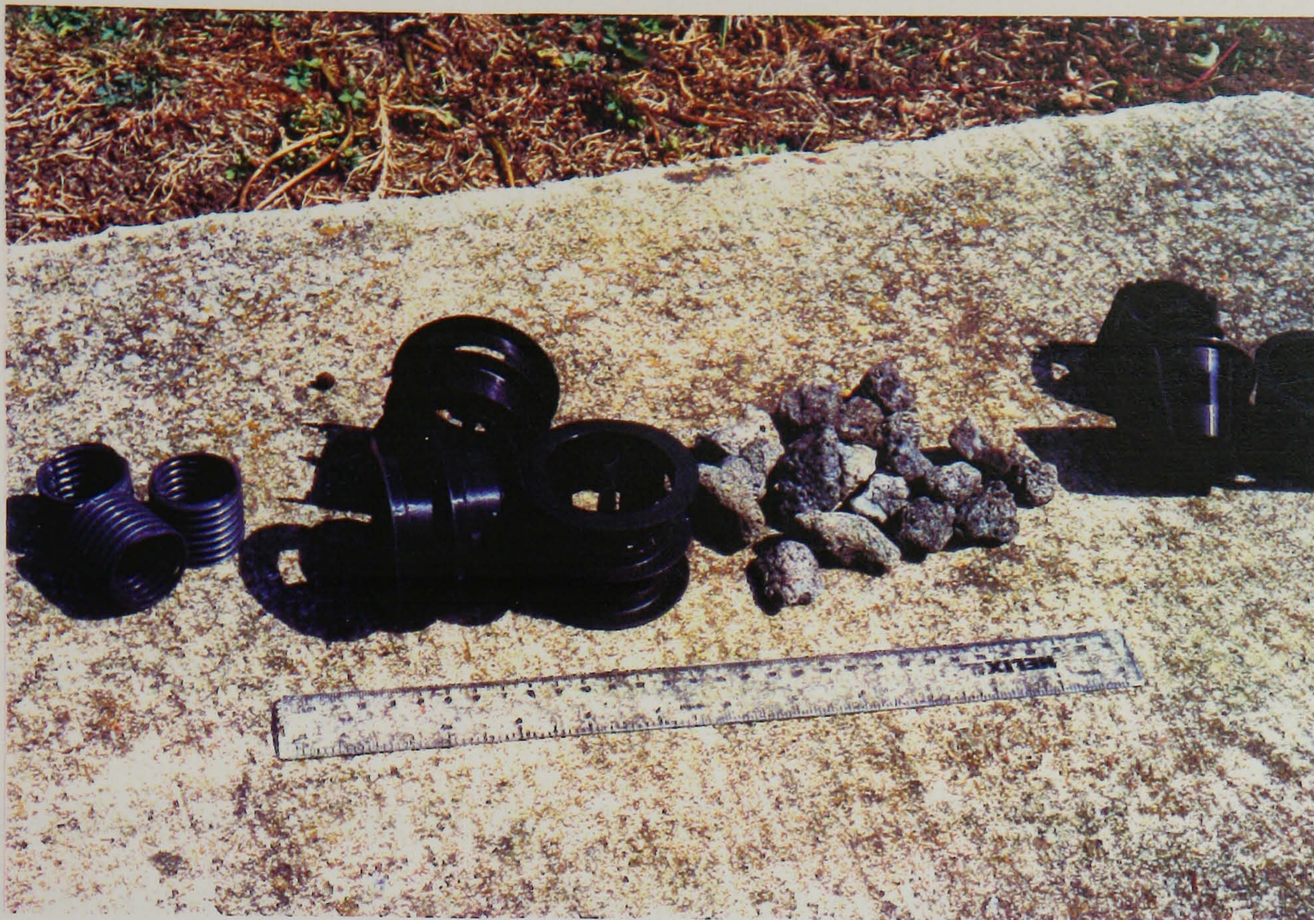
Plate 2: The media used in the pilot scale filters
