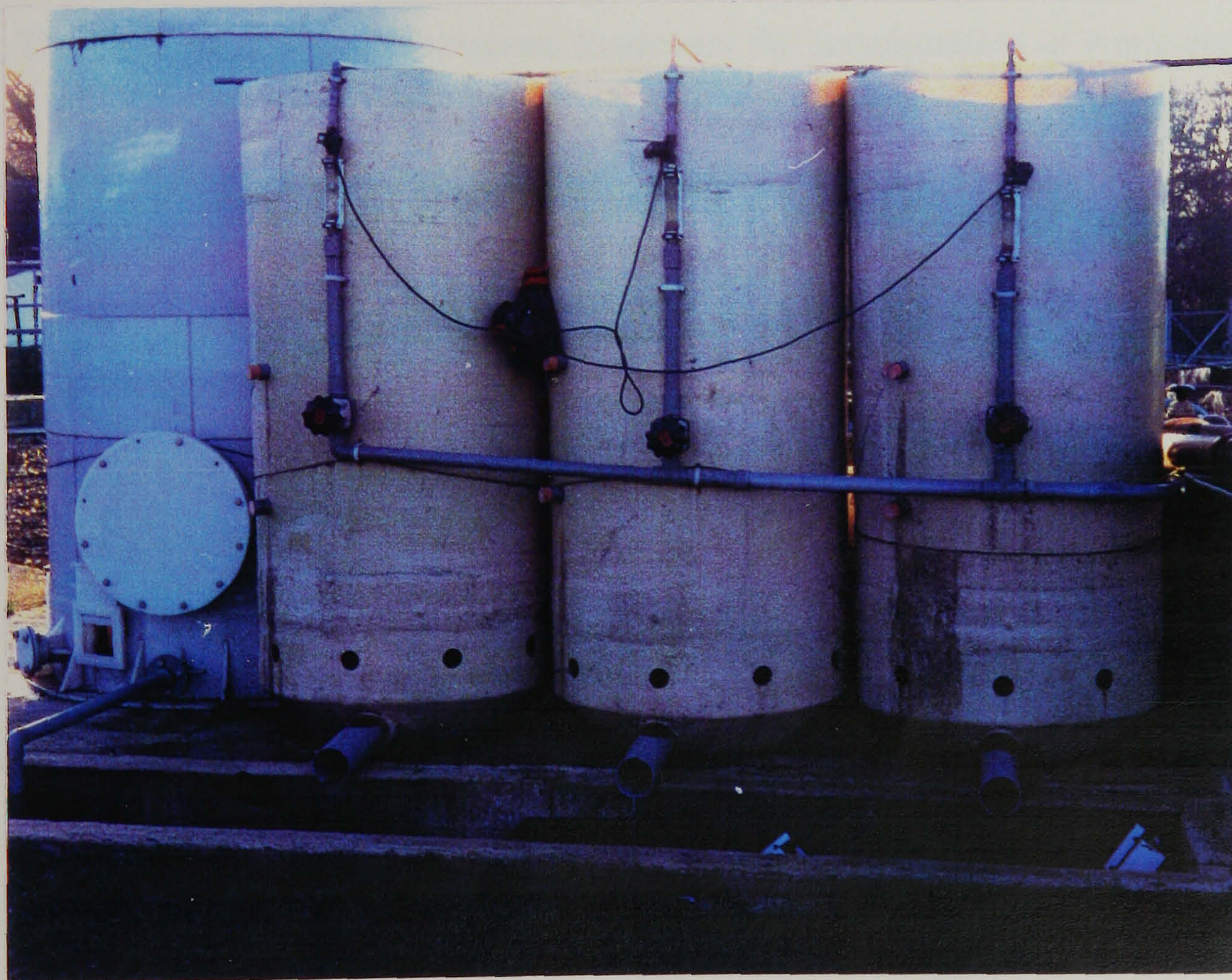
Plate 1: Pilot scale trickling filters
