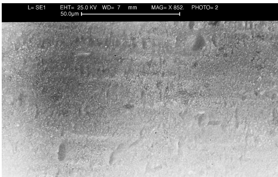
Figure 2.10 Electron micrograph of an o -phenylenediamine insulated electrode (Barton et al. , 2004).
