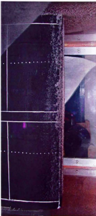
Figures 1 a & b. Ice formation in leading edge of a wing in the Cranfield University Icing Tunnel and in the engine inlet and rotor of an aircraft (NASA Glenn).
