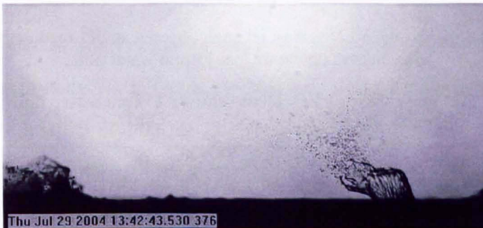
Figure 73. Corona top is swept by the airflow.
