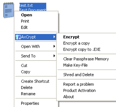
Figure 8: AxCrypt and Windows Explorer right click integration providing the option for encryption and decryption.
