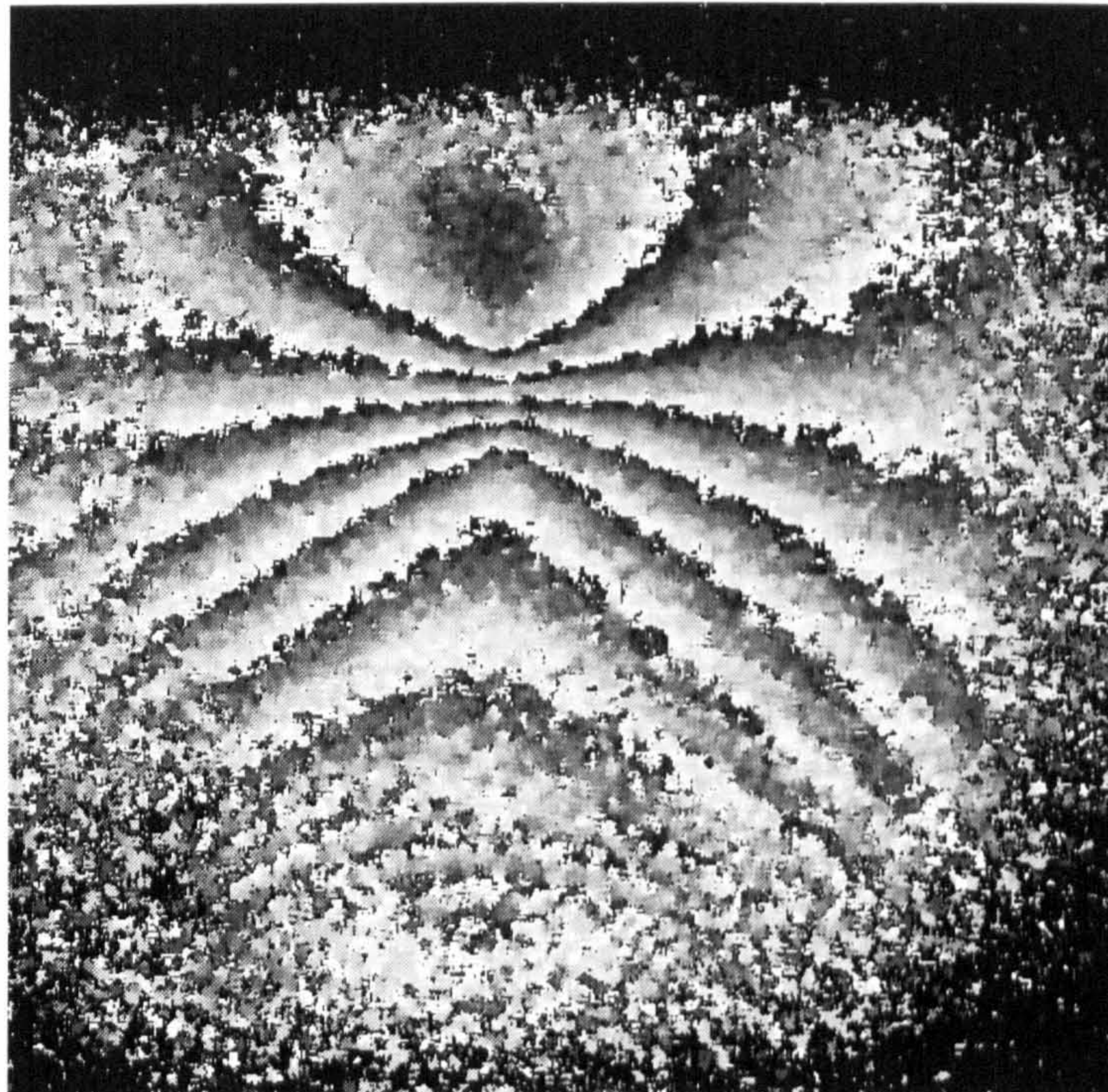
Figure 45 A shearography wrapped phase map from a mechanically loaded flat aluminium plate measuring 150mm by 180mm, with 10mm of vertical shear applied
