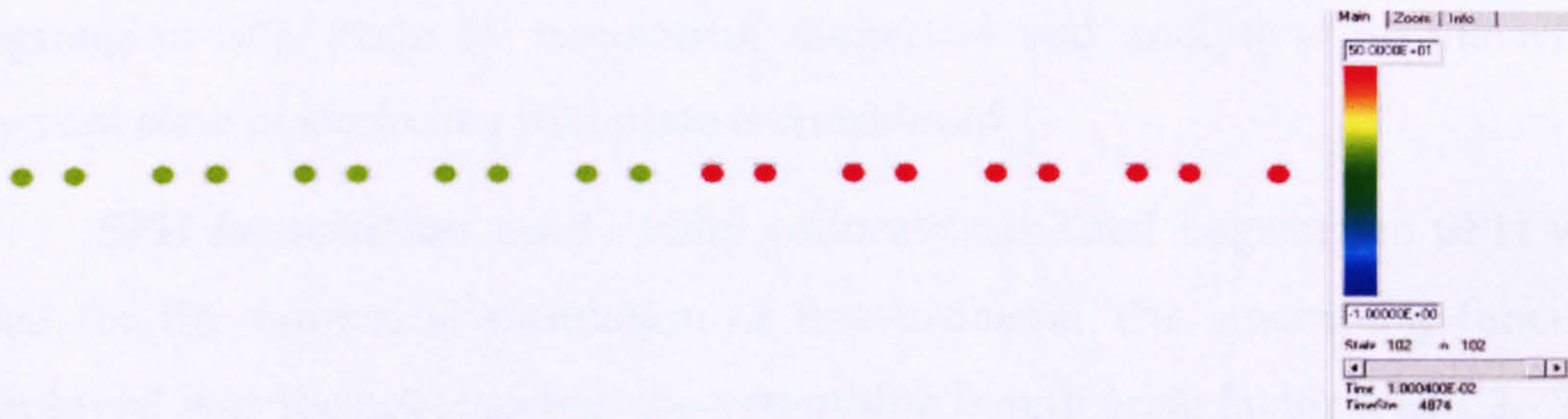
Fig. 6.1 Problem 1. Particles clump with specimen under tension, Eulerian Kernel. Only a few particles are shown.
