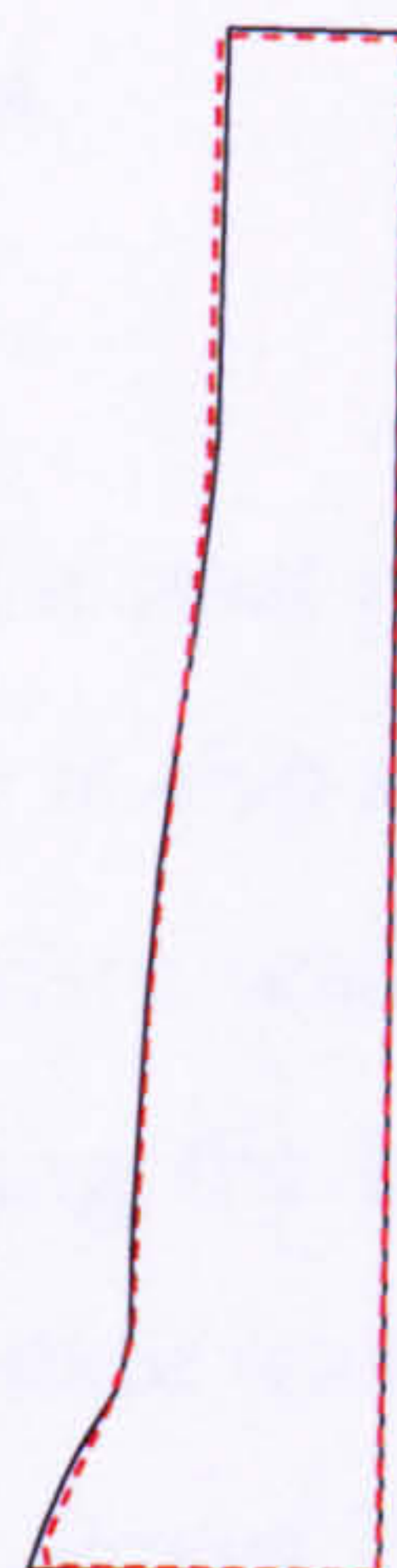
Fig 6.20. Problem 6. SPH vs FE final profile comparison, 2-D Taylor test (SPH=Solid line, FE=Dashed line)
