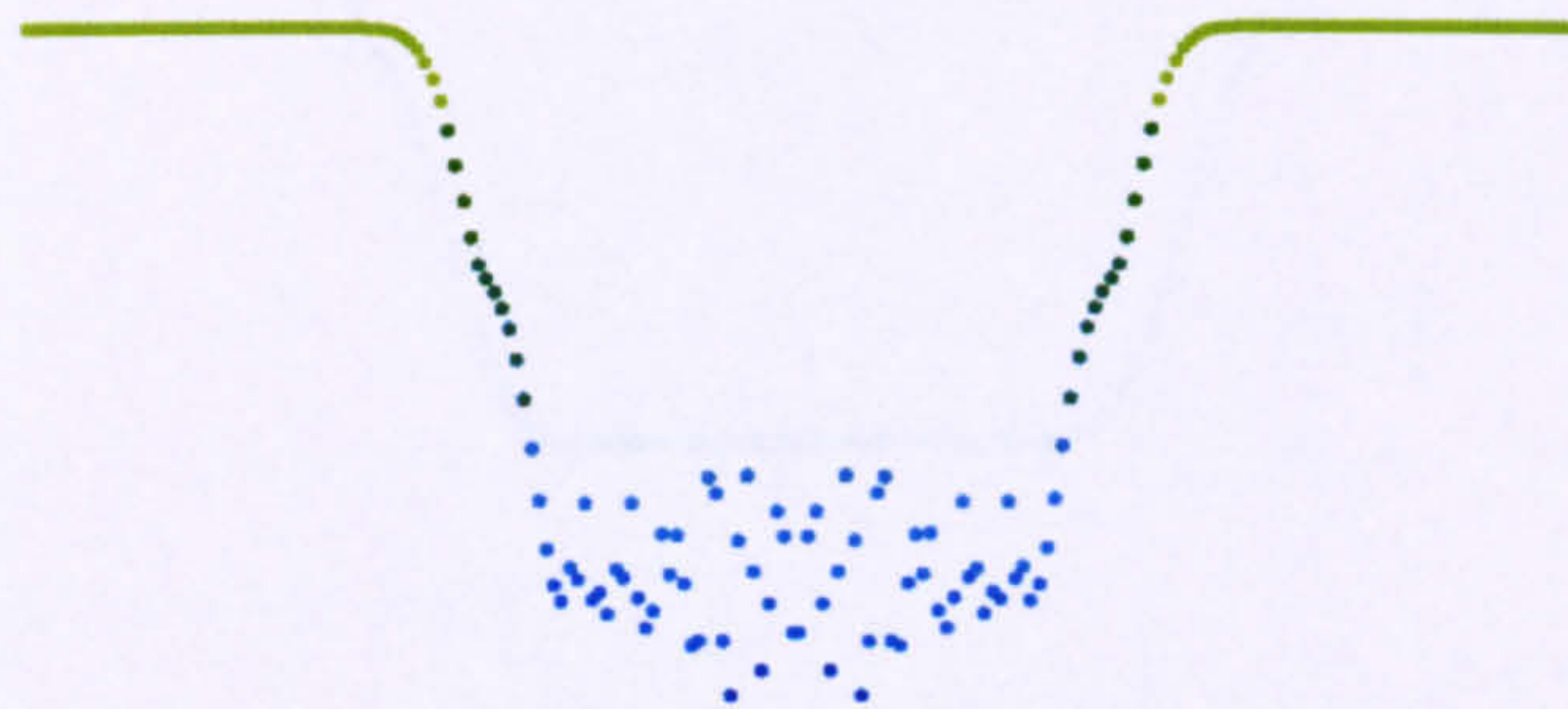
Fig. 7.7 Compressive wave, no artificial viscosity term in momentum equation
