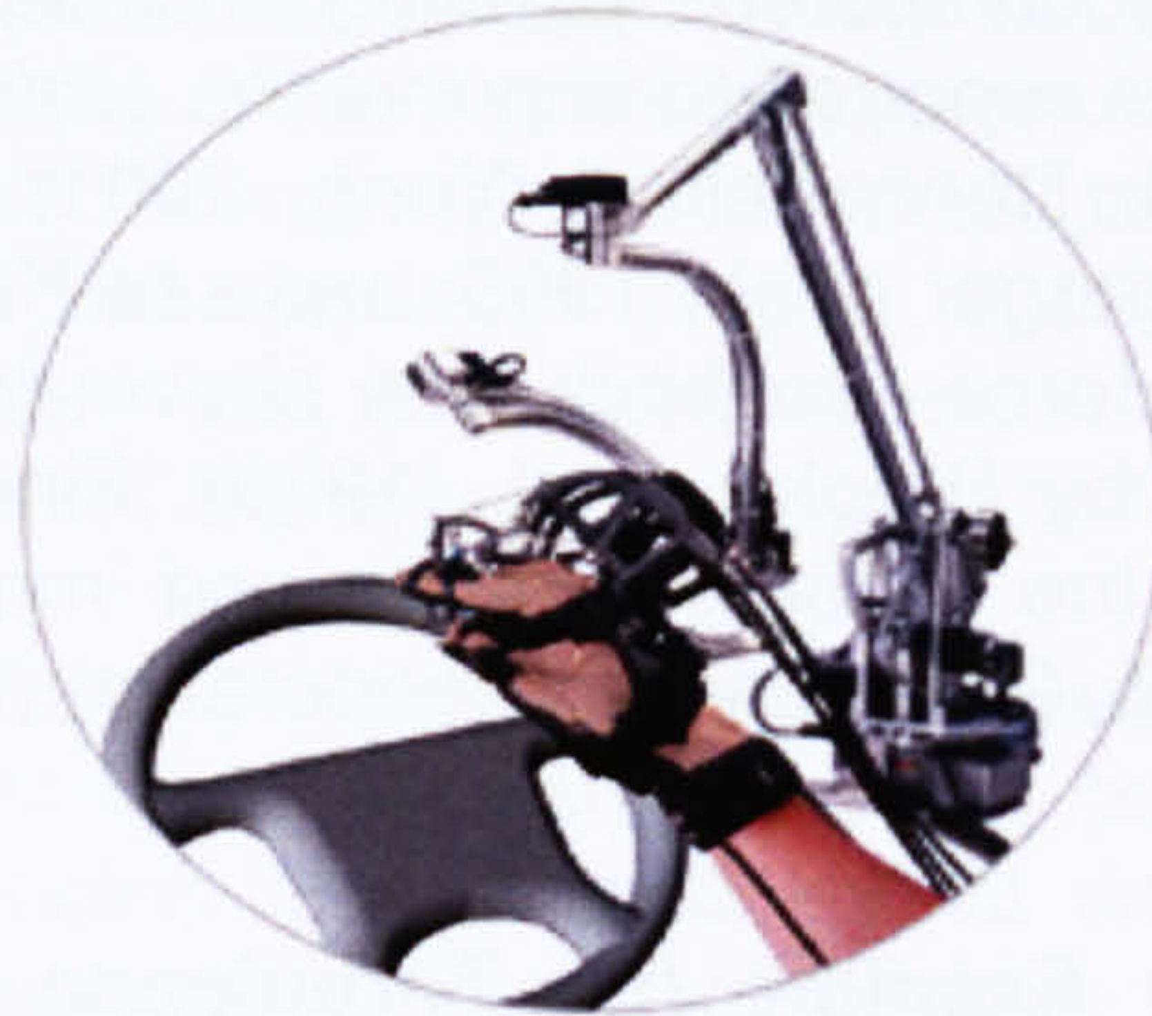
Figure 5: CyberForce attached to the CyberGlove and CyberGrasp system (Reproduced by permission of Immersion Corporation, Copyright © 2008 Immersion Corporation. All rights reserved)
