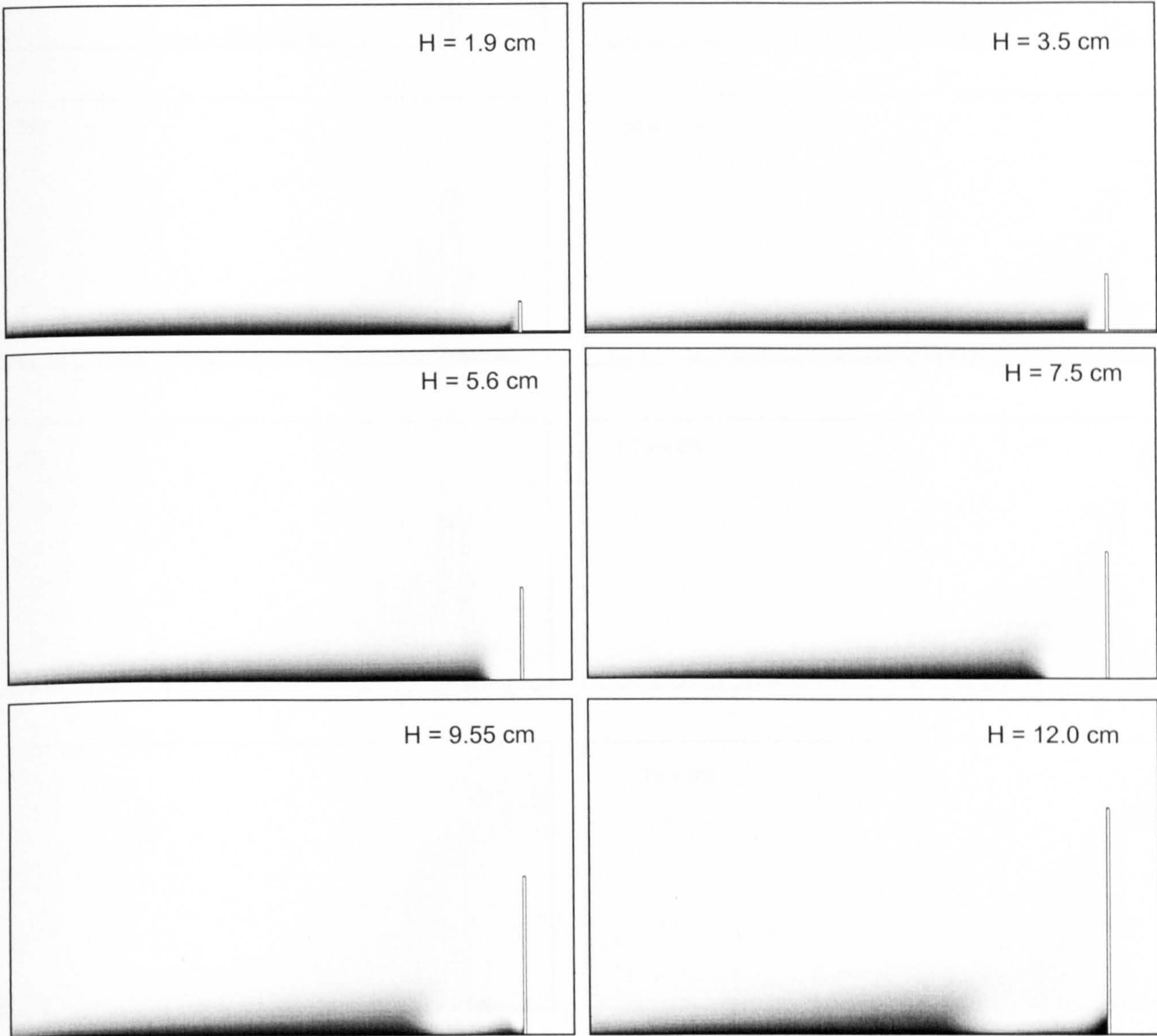
Figure 7.2: Early deposition stages in front of solid walls of different heights.
