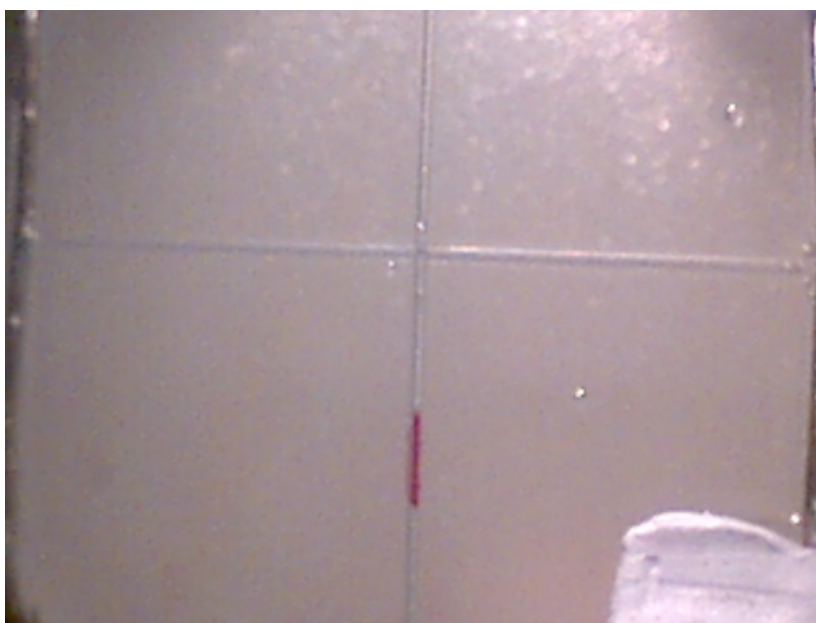
Figure 69: Injection of Rhodamine B into the dye channel.
