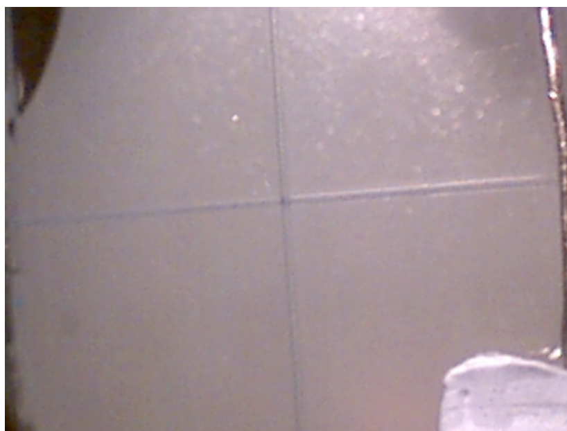
Figure 68: Capillary T-junction in Perspex.
