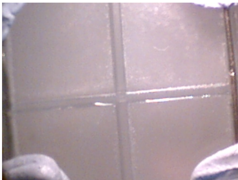
Figure 65: T-Junction drilled in Perspex
