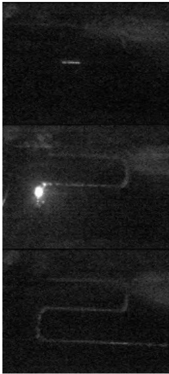
Figure 80: Successive images taken with a CCD camera in the dark under the illumination of a UV light during the scanning of an S-shaped channel in which Rhodamine B flows
