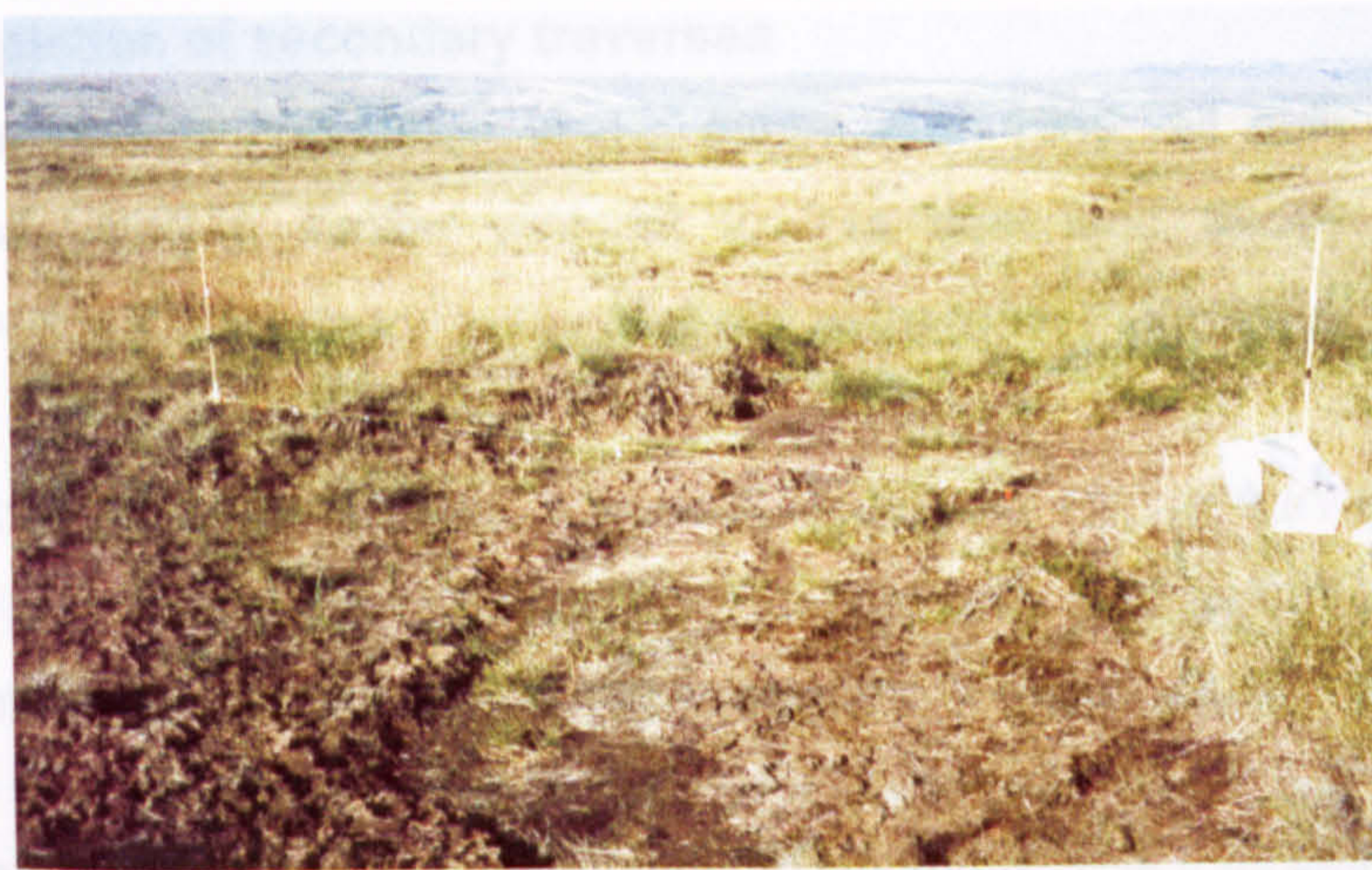
Plate 4.3 Traverse tape stretched across shallow erosion gully. The observation points at 25 cm intervals on the traverse tape can be seen as a series of coloured markers (Peak District).
