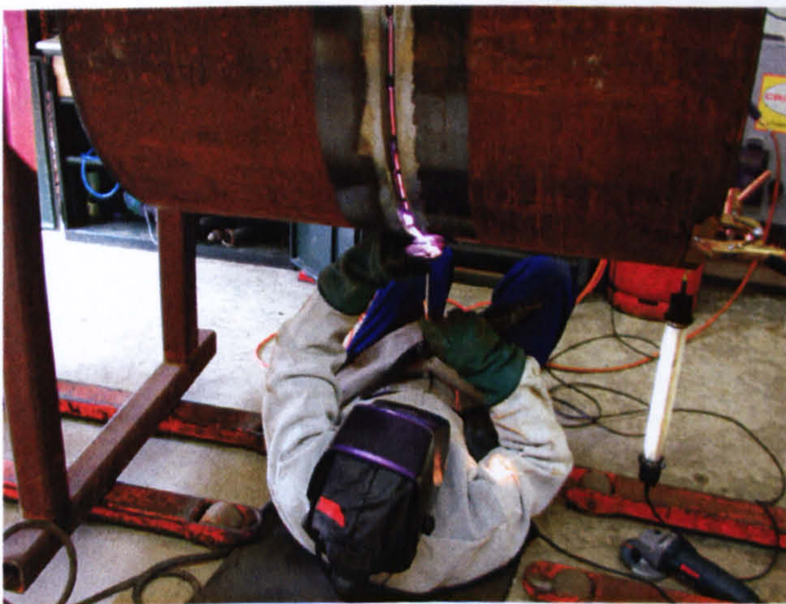
Figure 5-12: Tie-in procedure welding
