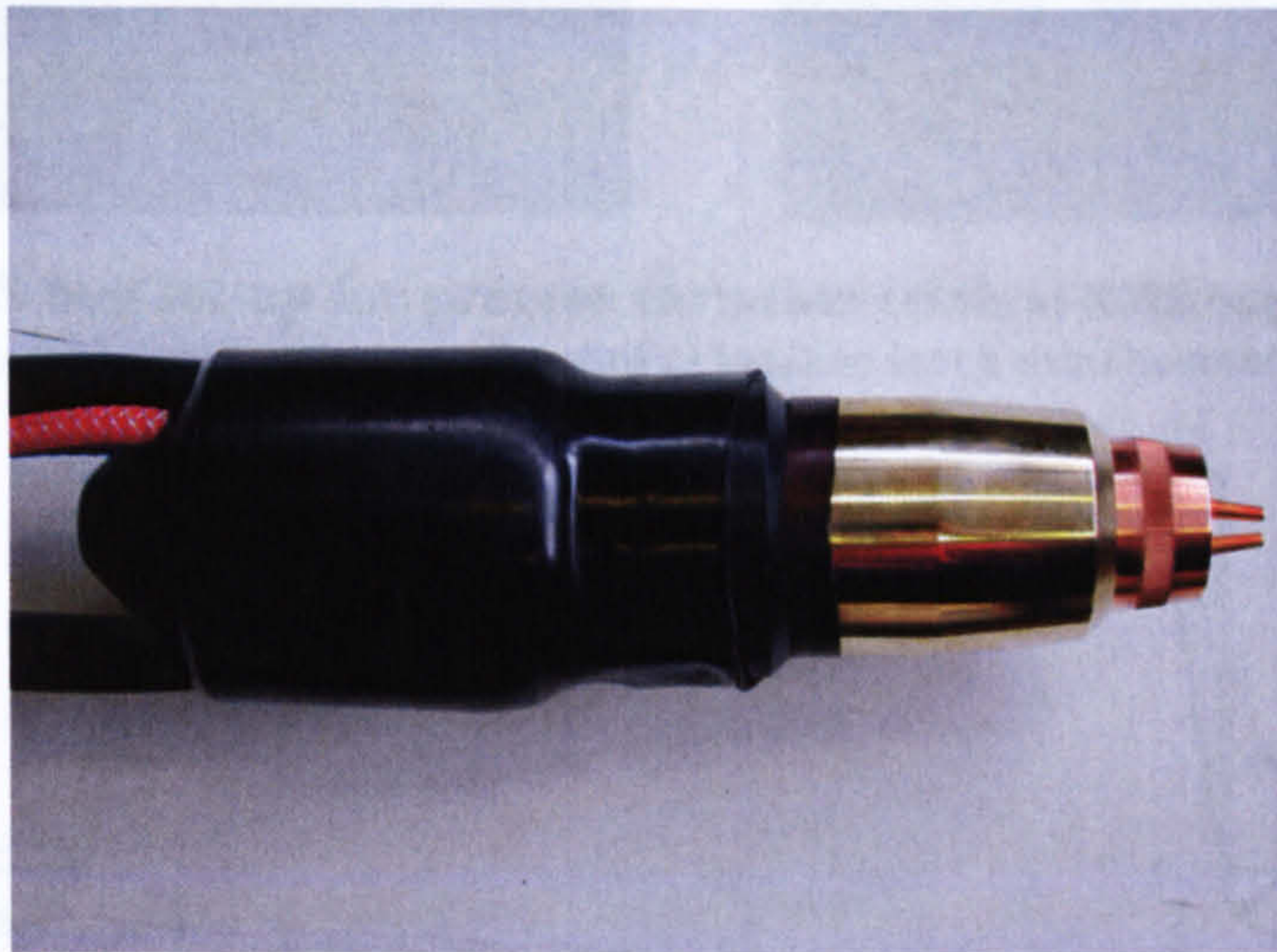
Figure 4-11: Water cooled WERC tandem torch
