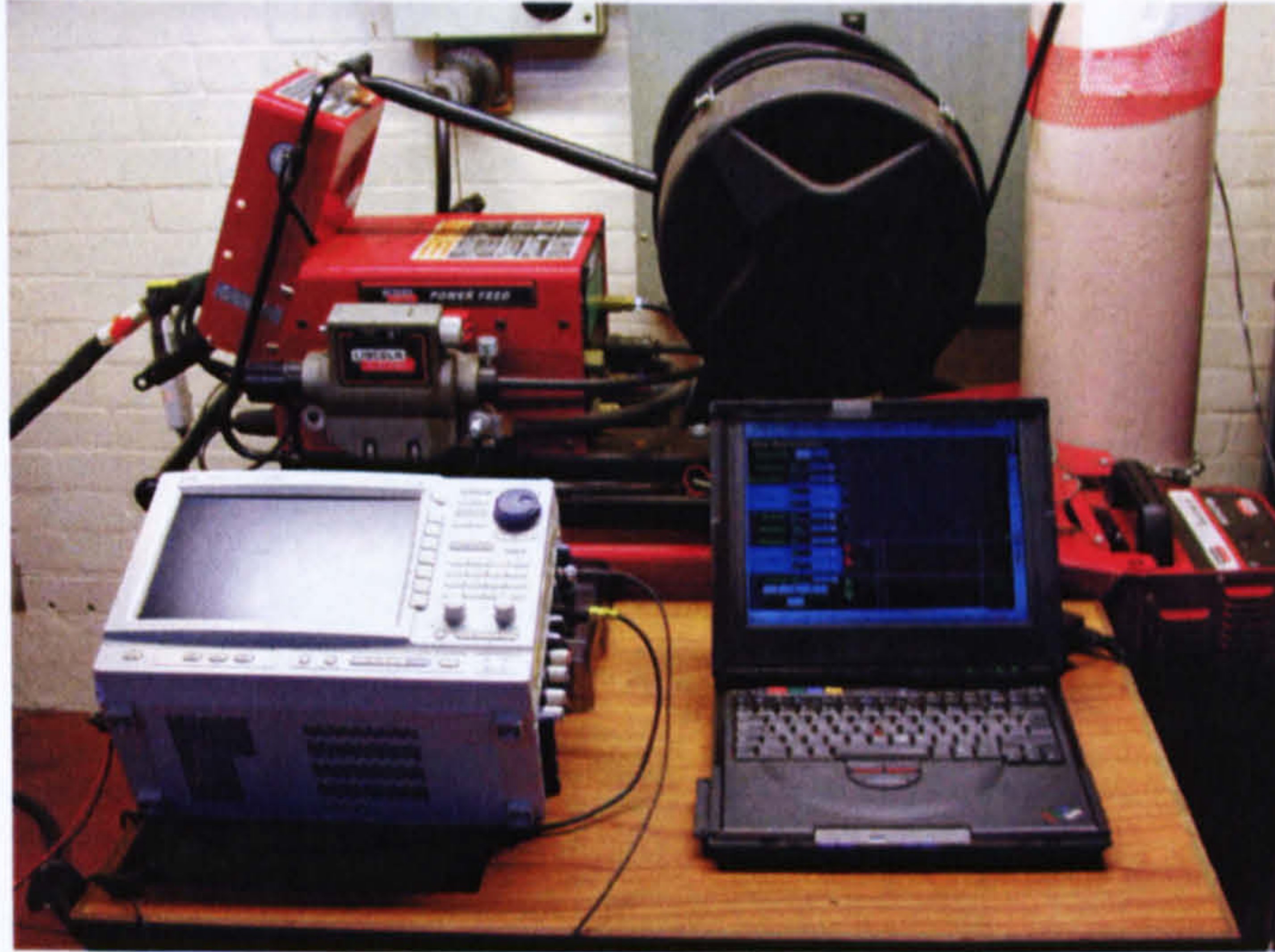
Figure 4-2: Narrow gap single wire welding power source (Lincoln 455 STT), Yokogawa Oscilloscope (DL 750) and Wavedesigner Pro ® power source control software
