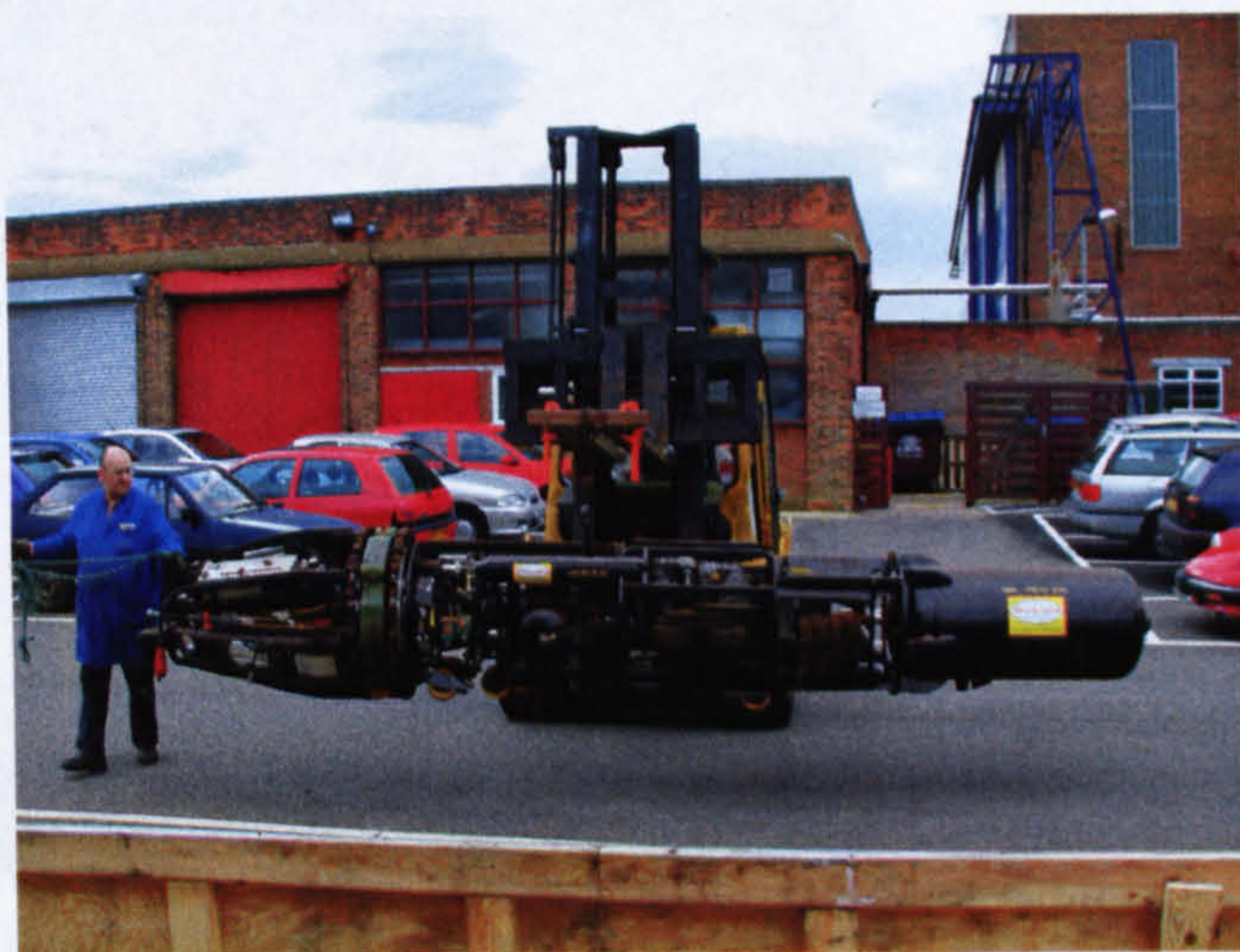
Figure 4-6: CRC-Evans 36 in. internal pipewelding machine
