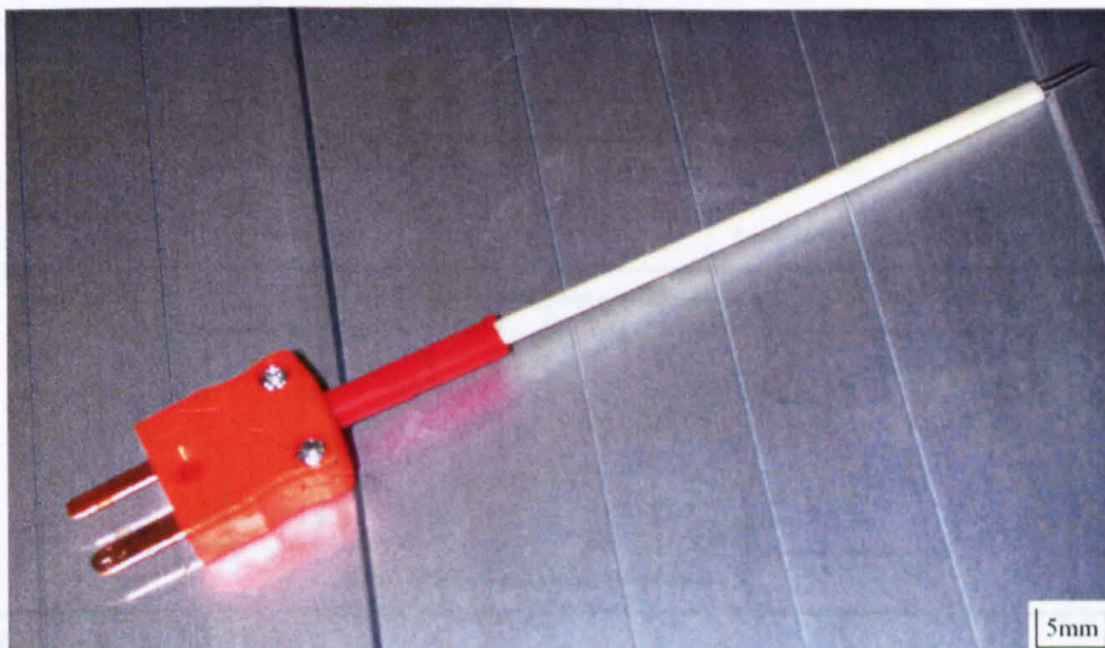
Figure 4-24: Externally placed thermocouple
