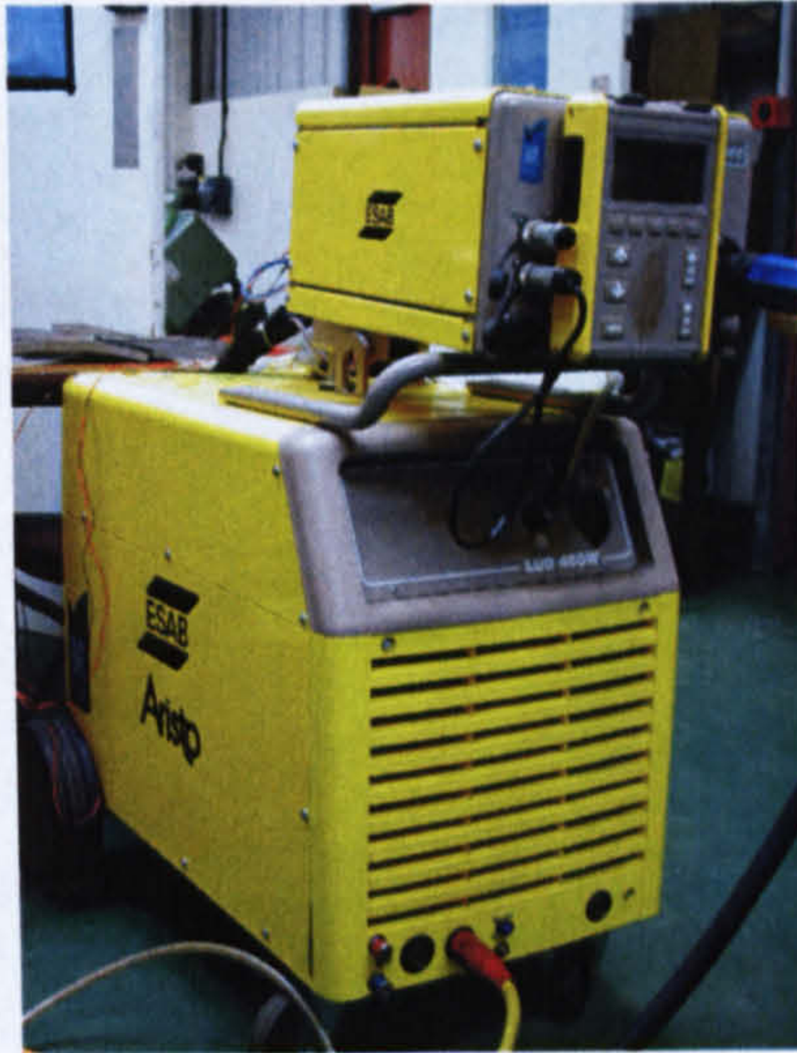
Figure 4-4: Tie-in and repair welding power source (ESAB Aristo 2000)
