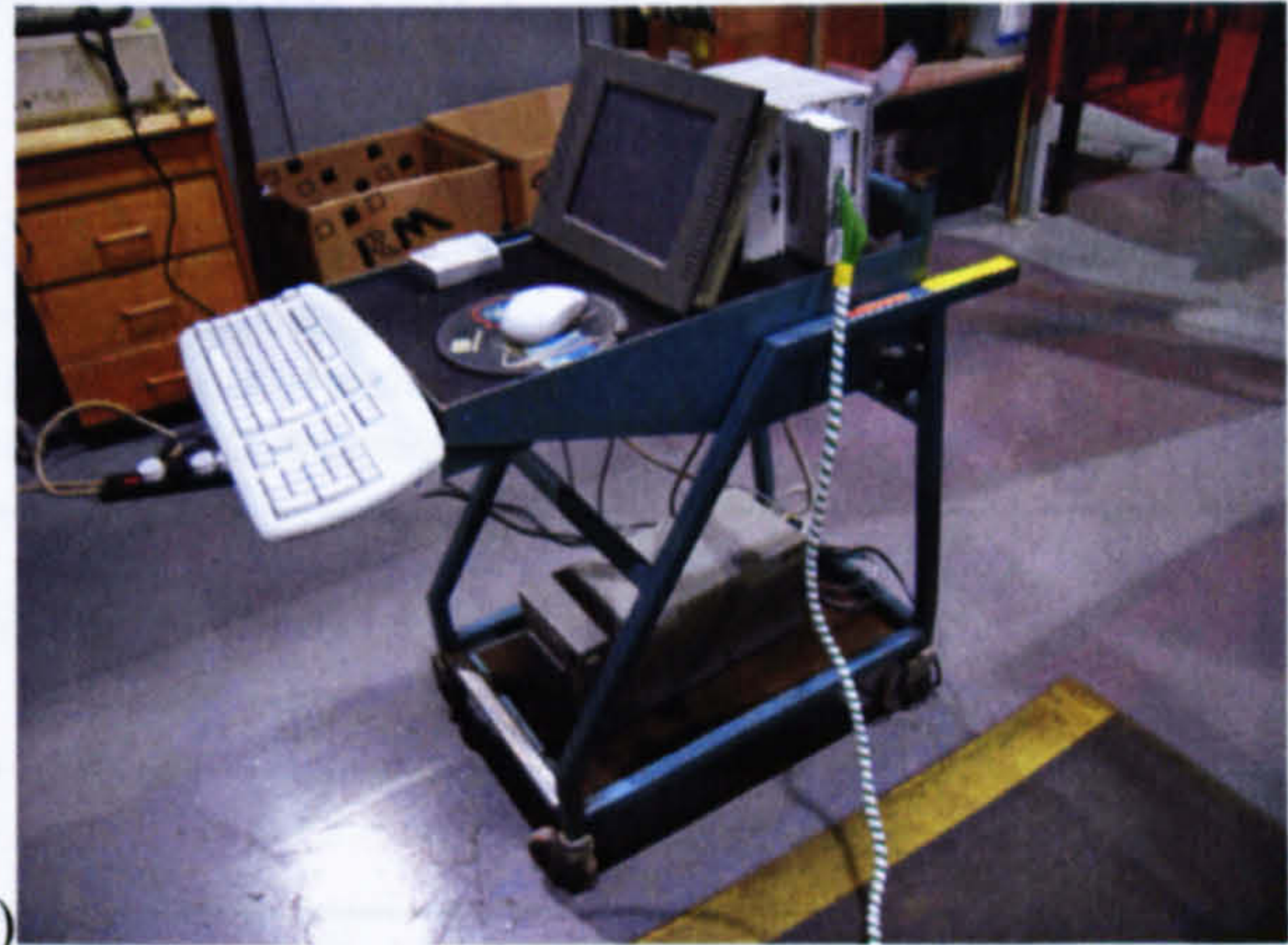
Figure 4-23: Thermocycle data capture equipment a) SCXI chassis unit and thermocouple module b) total thermocycle capture equipment (industrial pc on lowest shelf)
