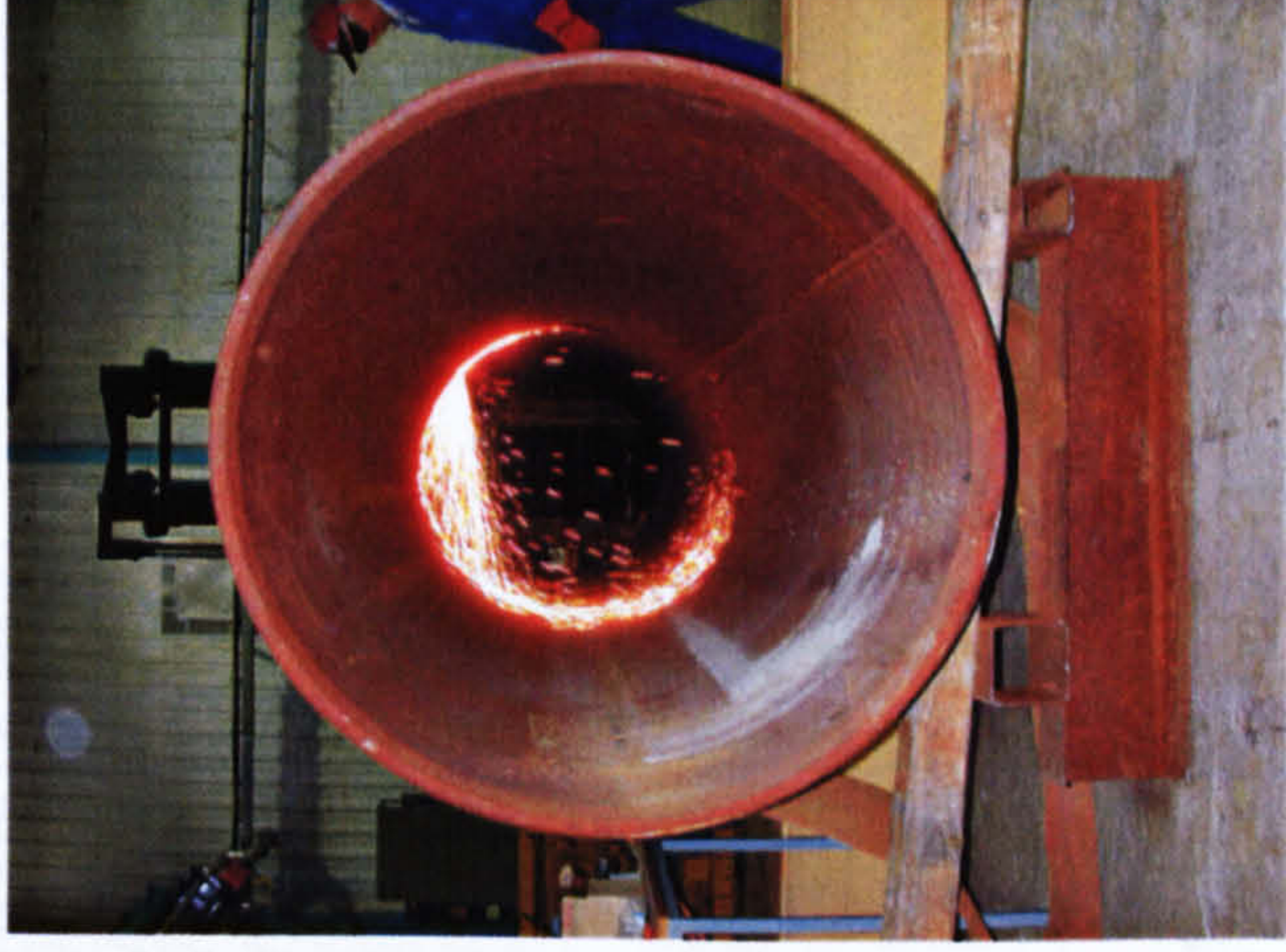
Mechanised oxy-acetylene cutting
