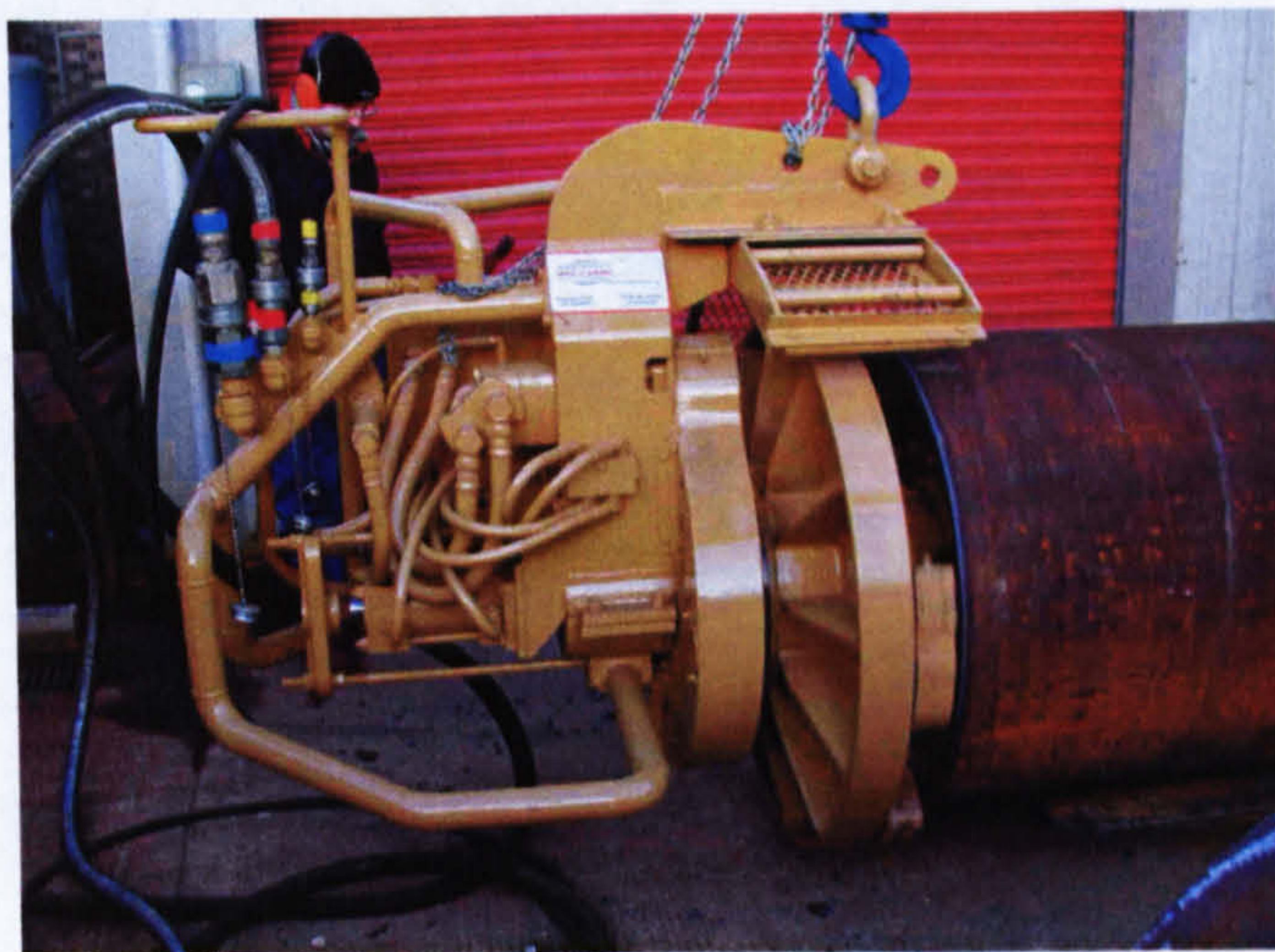
Figure 4-5: CRC-Evans 36 in. pipe facing machine
