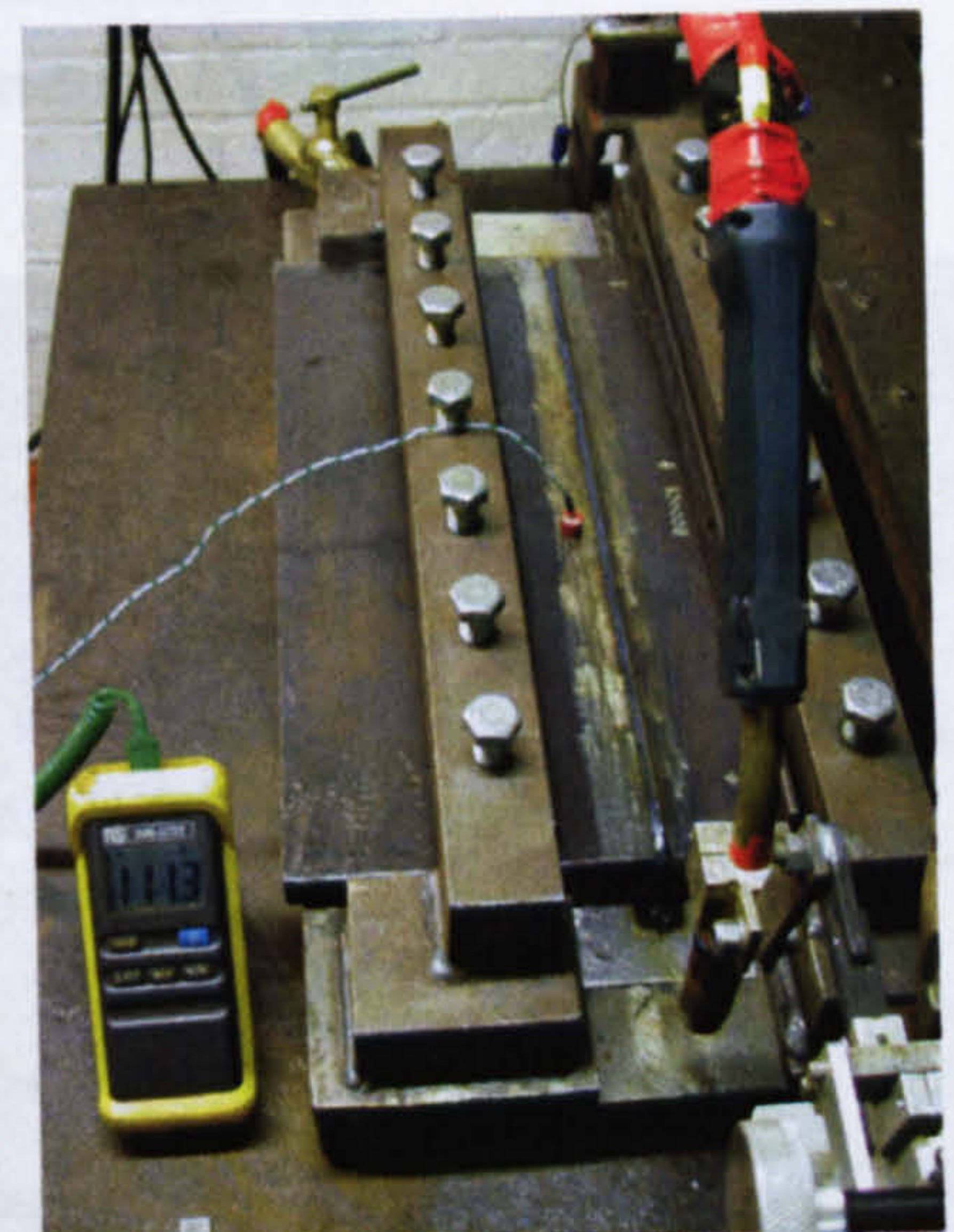
Figure 4-9: Equipment setup for flat plate welding
