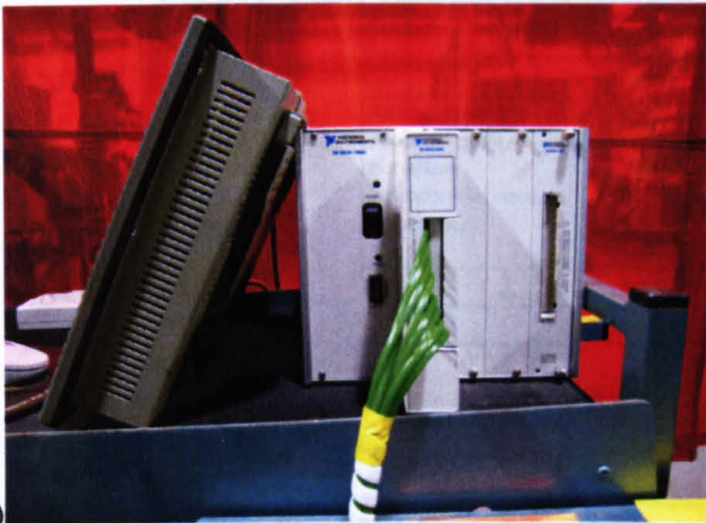
Figure 4-23: Thermocycle data capture equipment a) SCXI chassis unit and thermocouple module b) total thermocycle capture equipment (industrial pc on lowest shelf)
