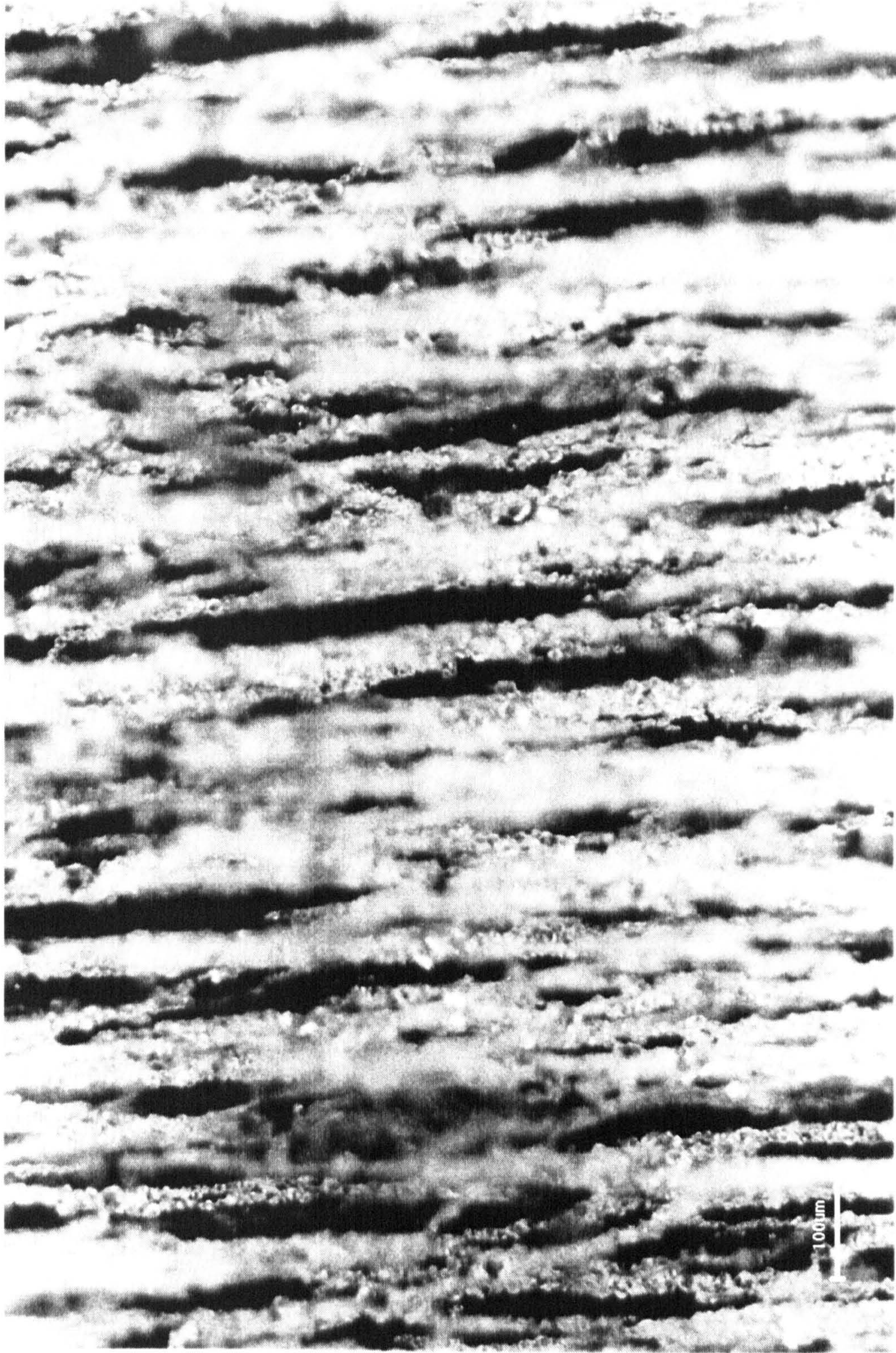
Figure 10.1 – ‘Pearl chains’ in a field-structured 10% vol. lead titanate / epoxy composite.
