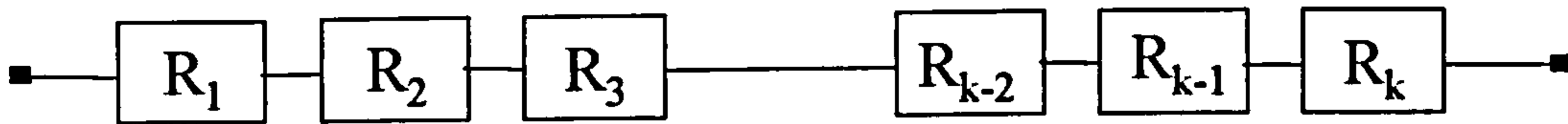
Figure 4.12 : Reliability Block Diagram of a Series System
