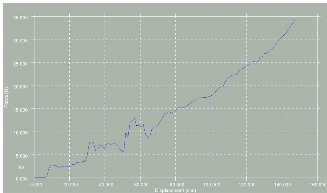
Figure 51 - Force displacement curve for Steel Frame (lateral impact).
