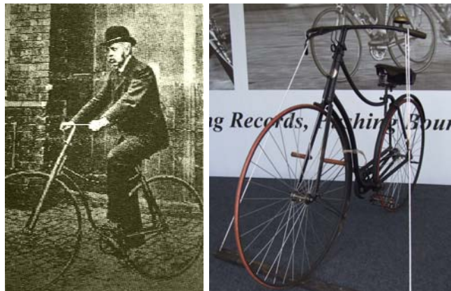
Figure 4 - J.K. Starley riding his Rover "Safety Bicycle" (courtesy British Cycle Industry Association / Goodwood collection)
