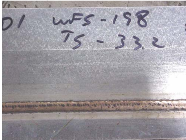
Figure 7. Spatter free GMAW-Pulse braze weld.
