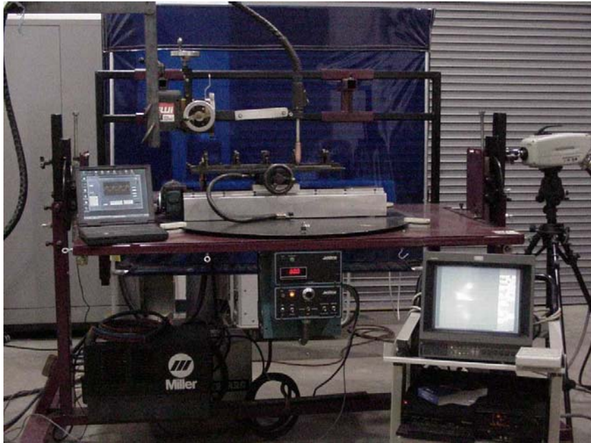
Figure 2. Welding table with stationary torch, high speed video, and data acquisition.
