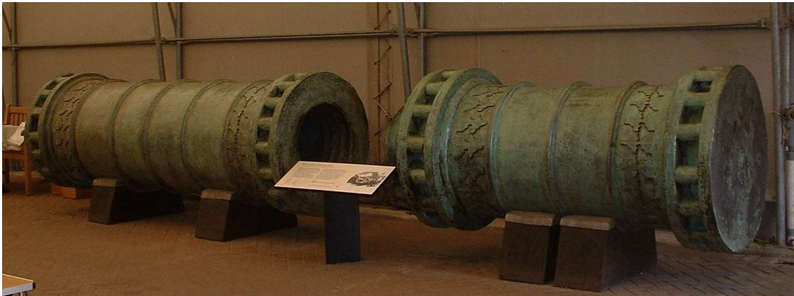
Figure 1.1: Turkish Bombard – given the relatively low density stone shot it fired, its thick wall is testament to its poor material utilisation (Public domain photograph taken at Royal Armouries, Fort Nelson, Portsmouth, England)
