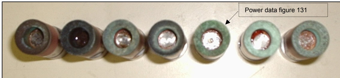
Figure 132 - Variation in wheel appearance after electro-discharge truing and then pre-process dressing the set of wheels
