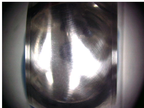
Figure 160 - Example of ball produced with an over-formed wheel. [#500 MRB-CBN, Elid 3]
