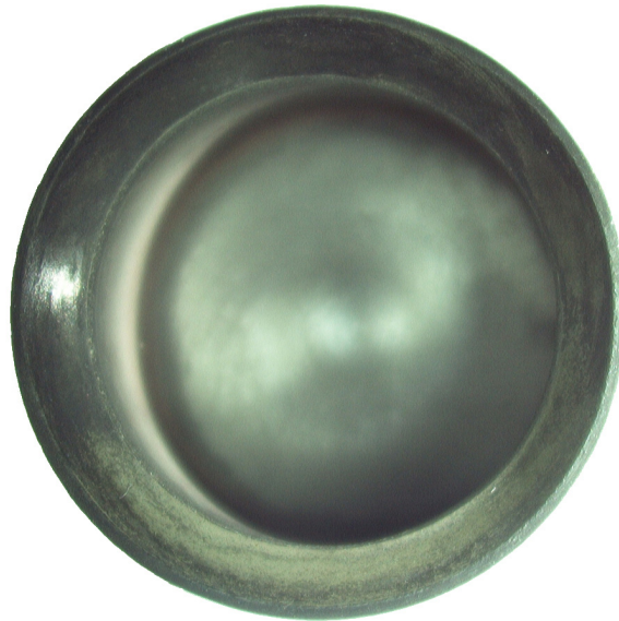
Appendix F4 - Example of a glazed wheel surface [#8000 MRB-CBN wheel]
