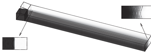
Figure 6: Computation of diffusion broadening in a microchannel using the characteristics-based Godunov-type scheme [4, 22].
