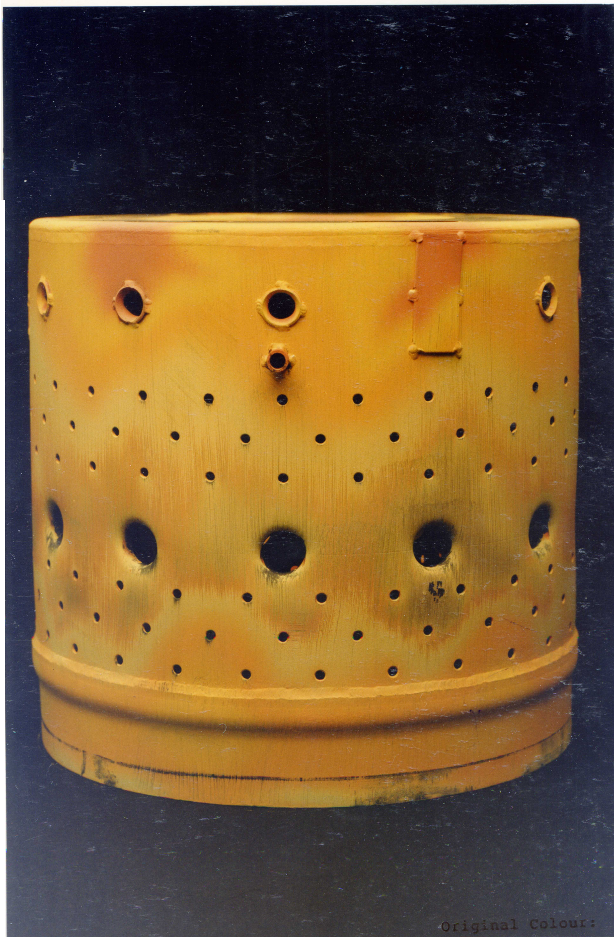
Plate 1: TEST LINER (CASE 3) - RUN WITH THERMAL PAINT
