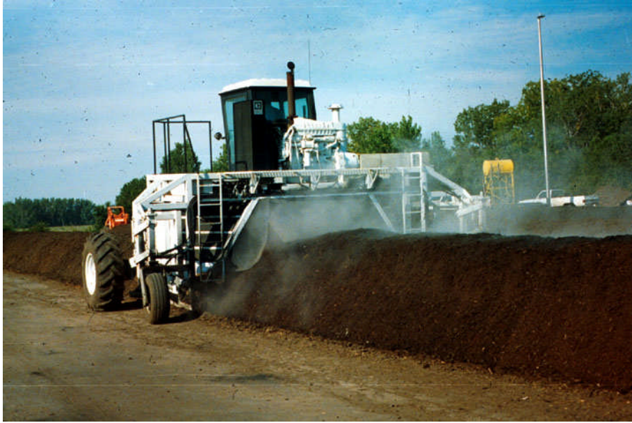
Figure 2.5 Windrow composting: turning the pile by a self-propelled machine.
