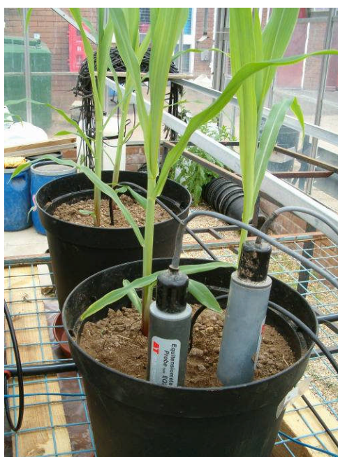
Figure A.3.2.2 Soil moisture control equipment.
