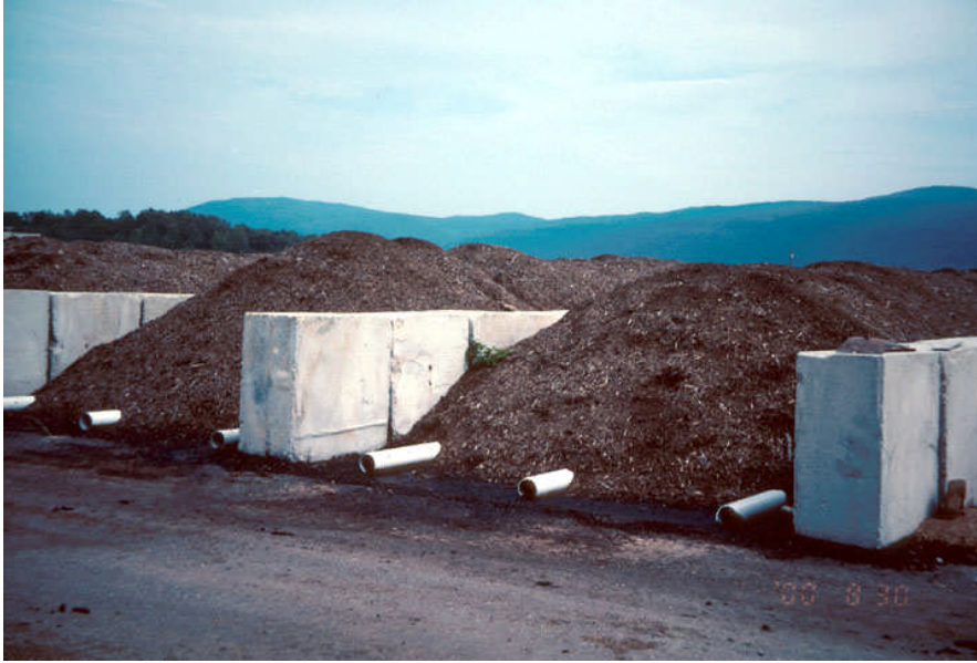
Figure 2.4 Static pile composting - passive aerated system.
