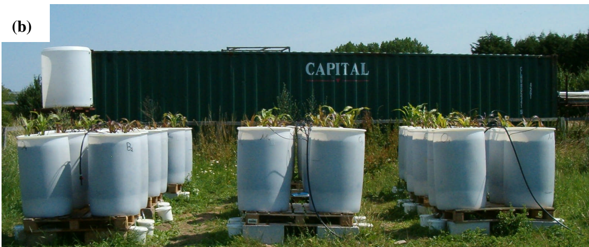
Figure A.3.3.4 View of the lysimeter trial on site: (a) before crop sowing (May 18) and (b) 5 weeks after crop emergence (July 12).
