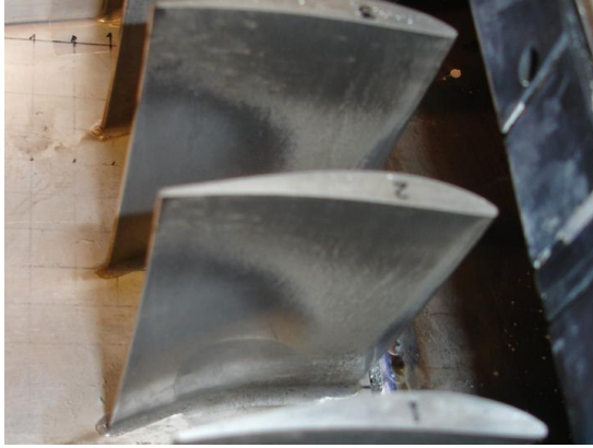
Figure 5-28 Results of pressure surface deposition after 3hr of real dust sample injection at rate of 100g/h.
