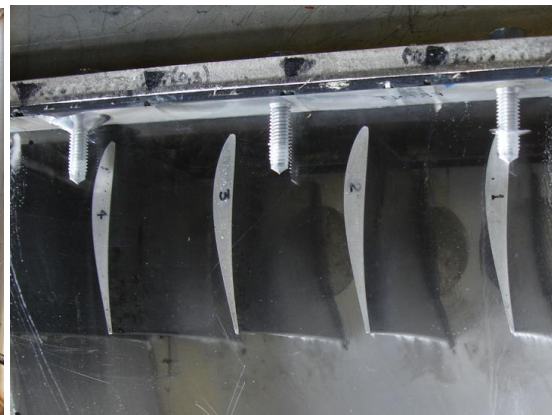
Figure 6-12 Top view of the cascade section during the washing on line process (test rig in operation).
