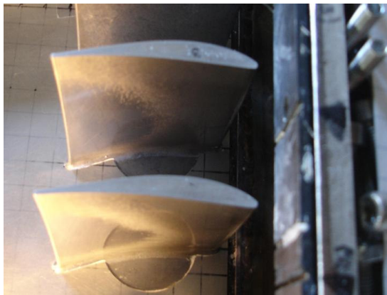
Figure 5-15 Results of pressure surface deposition after 4hr of artificial powder injection at rate of 100g/h.
