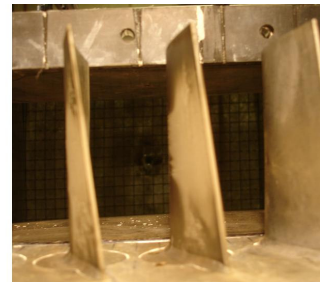
Figure 5-40. Results of pressure surface deposition after 5hr of real dust sample injection at rate of 100g/h.
