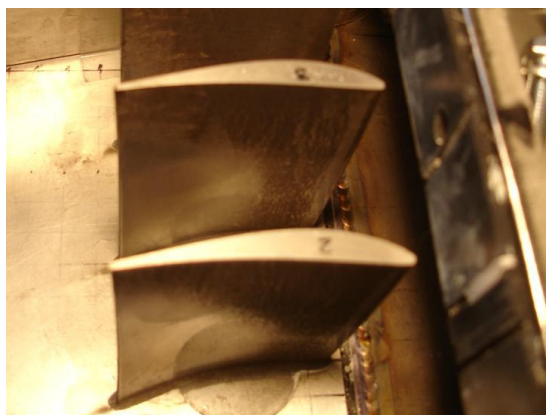
Figure 5-26 Results of pressure surface deposition after 2hr of real dust sample injection at rate of 100g/h.
