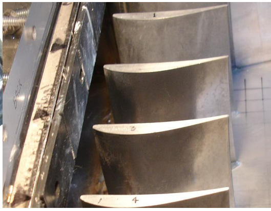
Figure 5-20 Results of suction surface deposition after 6hr of artificial powder injection at rate of 100g/h.
