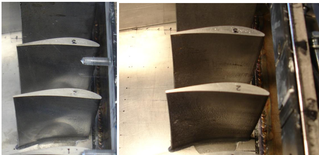
Figure 6-15 Pressure surface of the blades after the washing process (left). Pressure surface of the blades after 1hour of dust injection at rate of 100g/hr equivalent to 1.5 day of engine operation (right).
