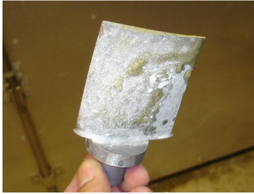
Figure 5-23 Test of liquid-grass as glue-agent in the deposition of artificial dust.
