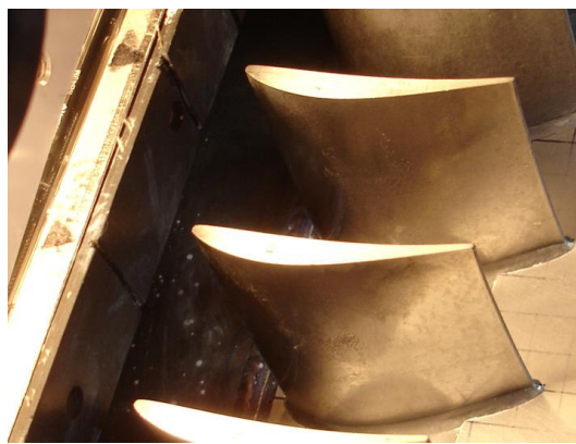
Figure 5-22 Results of suction surface deposition after 7hr of artificial powder injection at rate of 100g/h.
