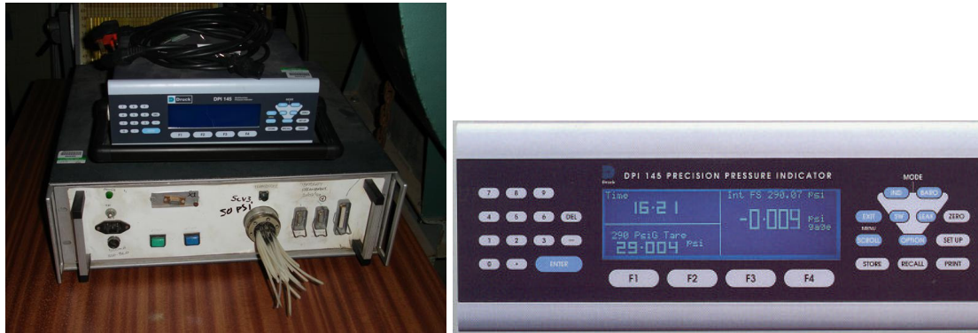
Figure 3-18 Pressure transducer and electronic display (left). Screen from the DRUCK electronic display (left). The electronic display had pressure ranges of up to 700 bar with a precision of 0.15 mbar.
