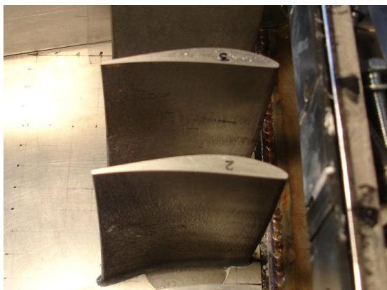
Figure 5-24 Results of pressure surface deposition after 1hr of real dust sample injection at rate of 100g/h.
