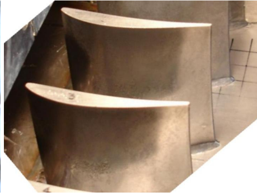
Figure 5-14 Results of suction surface deposition after 3hr of artificial powder injection at rate of 100g/h.
