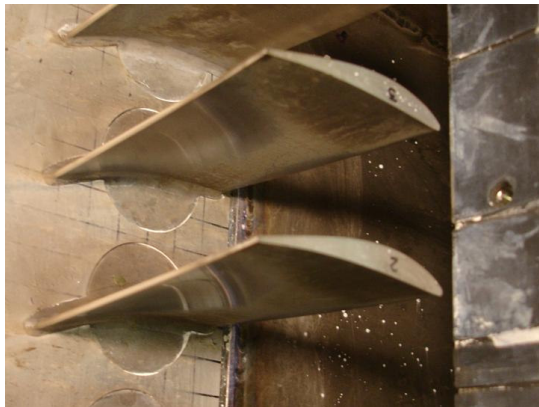
Figure 5-32 Results of pressure surface deposition after 5hr of real dust sample injection at rate of 100g/h.
