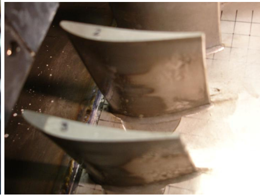
Figure 5-29 Results of suction surface deposition after 3hr of artificial dust injection at rate of 100g/h.
