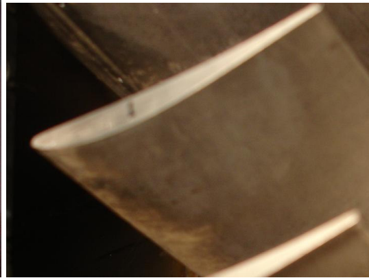
Figure 5-42 Experimental result of fouling on the suction surface after 1hr of artificial dust injection at rate of 100g/h.
