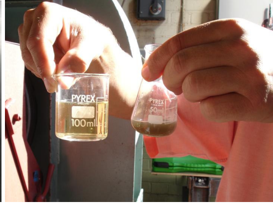
Figure 6-14 Washing-fluid before the cleaning process (left). Washing-fluid collected from the cascade (right).
