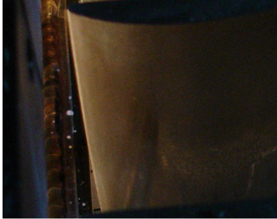
Figure 5-7 Artificial powder deposition on the leading edge (suction surface) after 7 hours of test rig operation (injection rate of 100g/hr).
