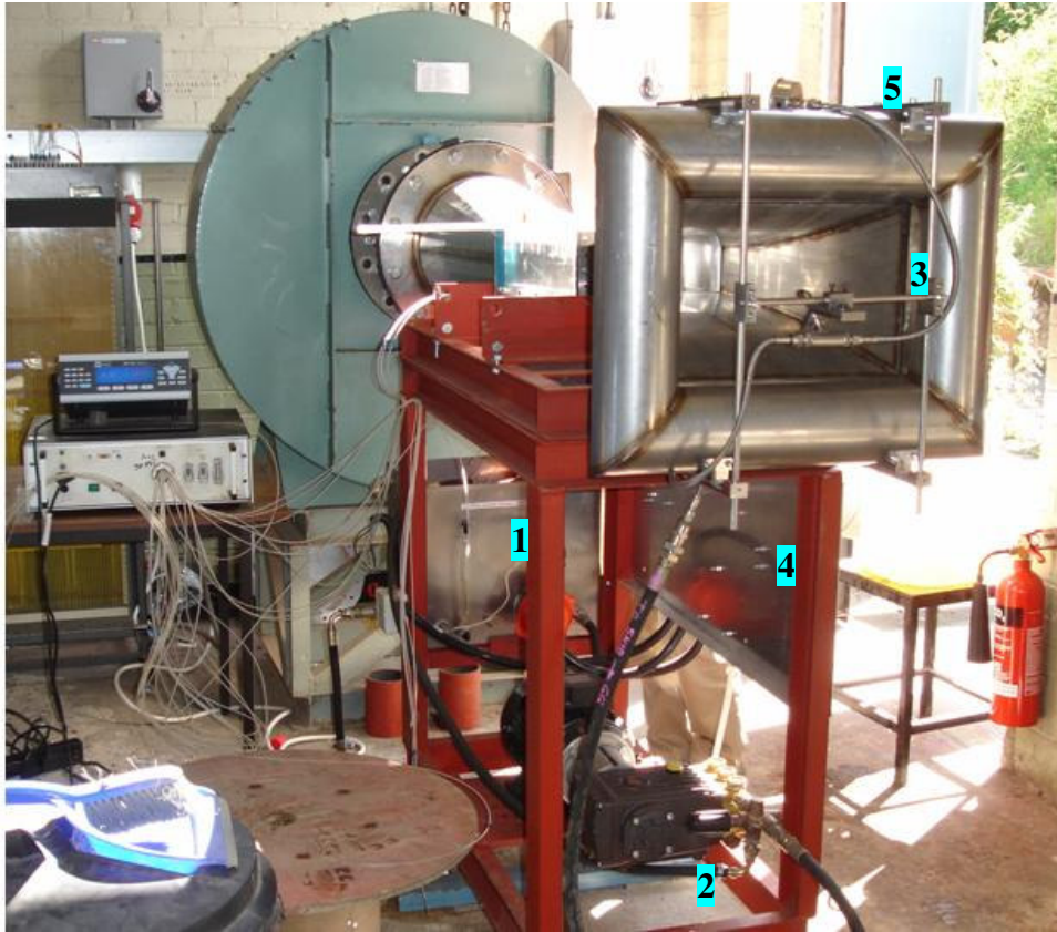
Figure 6-10. Compressor washing system installed in the test rig.
