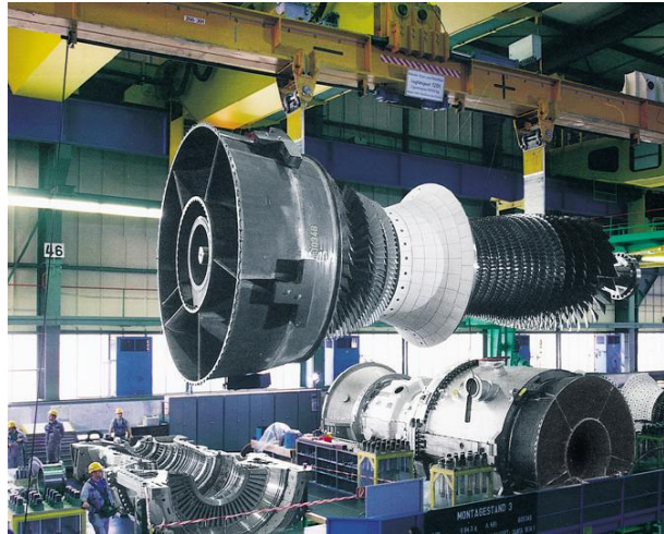
Gas Turbine model SIEMENS V94.3A (Siemens (2005)).
