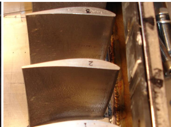
Figure 5-46 Experimental result of fouling on the suction surface after 7hr of dust injection at rate of 100g/h.
