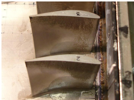
Figure 5-36 Results of pressure surface deposition after 7hr of real dust sample injection at rate of 100g/h.
