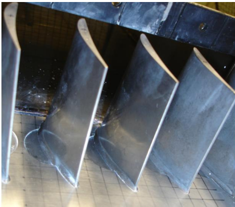
Figure 5-5 Artificial powder deposition on suction surface after 7 hours of test rig operation (injection rate of 100g/hr).
