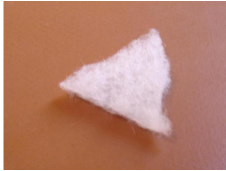
Figure 3-14 Sample of the cloth-filter: efficiency of 90% for particles retention of 10 \mu m, synthetic fiber media thickness of 10mm and pressure drop of 1% at low speeds (static filter).
