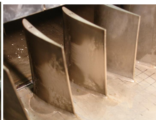
Figure 5-37 Results of suction surface deposition after 7hr of artificial dust injection at rate of 100g/h.
