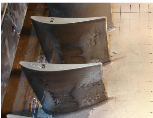
Figure 5-27 Results of suction surface deposition after 2hr of artificial dust injection at rate of 100g/h.
