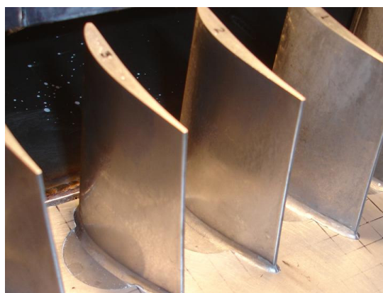
Figure 5-25 Results of suction surface deposition after 1hr of artificial dust injection at rate of 100g/h.
