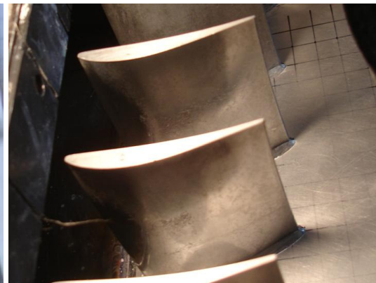
Figure 5-18 Results of suction surface deposition after 5hr of artificial powder injection at rate of 100g/h.
