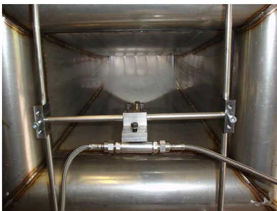
Figure 6-11 Compressor washing on line operating in the test rig.
