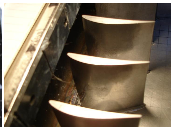
Figure 5-12 Results of suction surface deposition after 2hr of artificial powder injection at rate of 100g/h.
