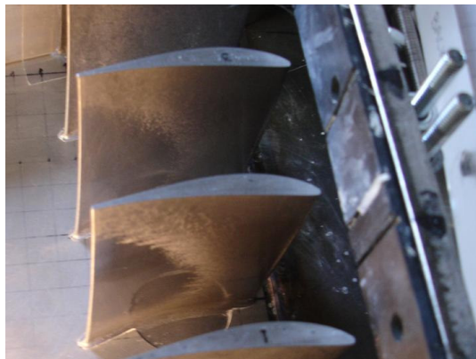
Figure 5-17 Results of pressure surface deposition after 5hr of artificial powder injection at rate of 100g/h.
