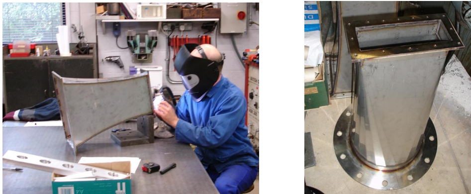
Figure 3-15 Manufacture of inlet-section (left) and outlet section (right) by the TIG welding process.
