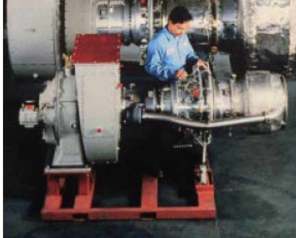
Photo-1 Gas Turbine model Saturn 20
