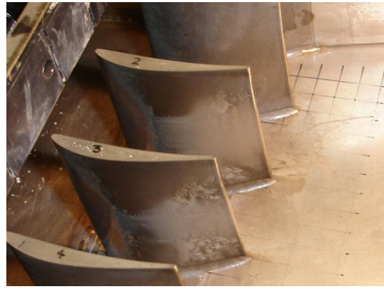
Figure 5-35 Results of suction surface deposition after 6hr of artificial dust injection at rate of 100g/h.
