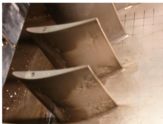
Figure 5-33 Results of suction surface deposition after 5hr of artificial dust injection at rate of 100g/h.
