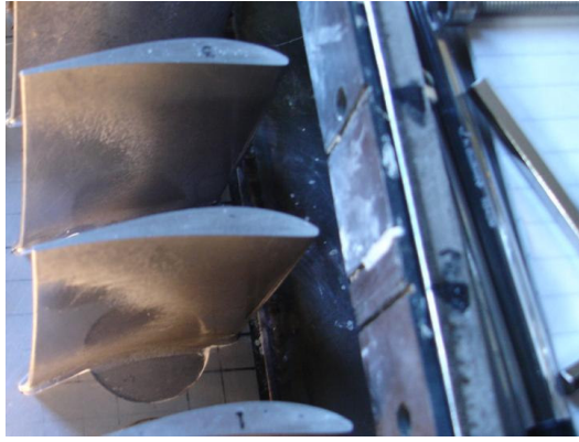
Figure 5-13 Results of pressure surface deposition after 3hr of artificial powder injection at rate of 100g/h.
