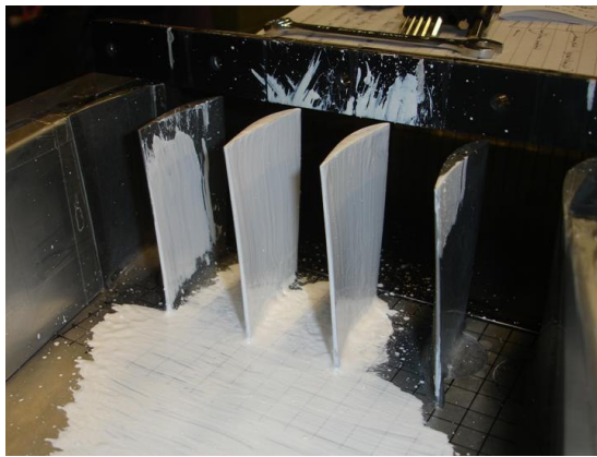
Figure 4-26 Application of mixture of TiO and Kerosene on blades to visualize the flow path (pressure surfaces).
