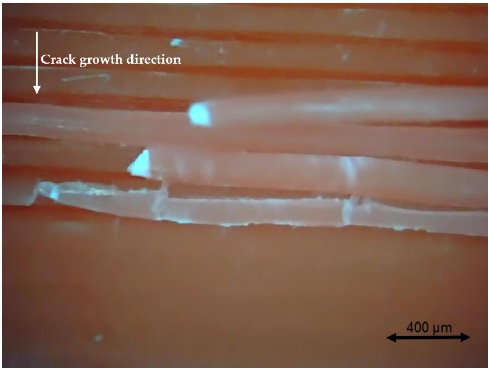
Figure 8-14 Specimen with a nozzle size of 0.8 mm, Y building orientation, and layer thickness of 0.15 mm.
