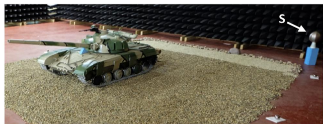
FIGURE 4 Target scene, consisting of a Quarter scale T72 tank model on gravel and reference sphere “S”.
