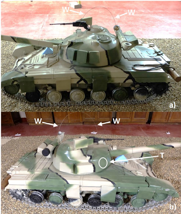
FIGURE 13 Close-up side-views of the quarter scale T72 tank model. The highlighted parts are the arched antenna wire “W”, and the bistatic specular reflection point on the turret “T”.
